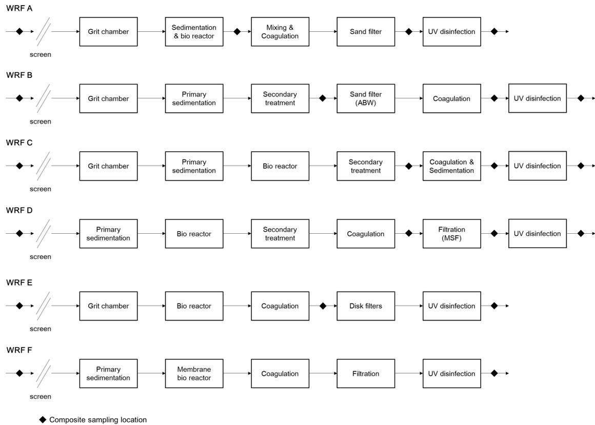
Fig. 1. Process flow diagrams of the six water reclamation facilities surveyed.
