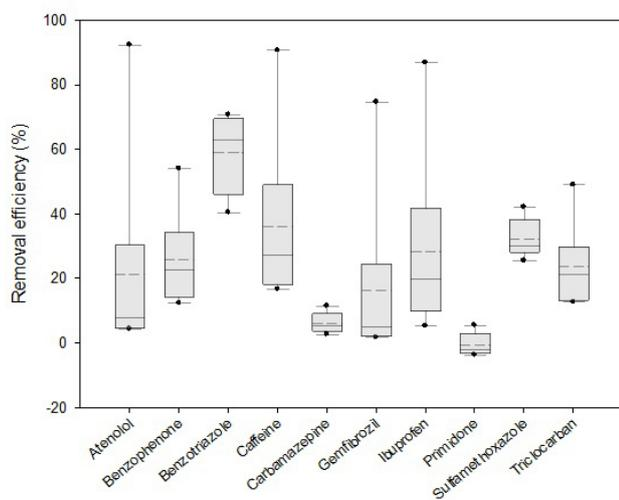
Fig. 4. Removal efficiencies of PPCPs by UV disinfection at six WRFs (A, B, C, D, E and F). (Box plot: 25th percentile, median, average and 75th percentile,  $\perp$ : 10th and 90th percentiles.)
