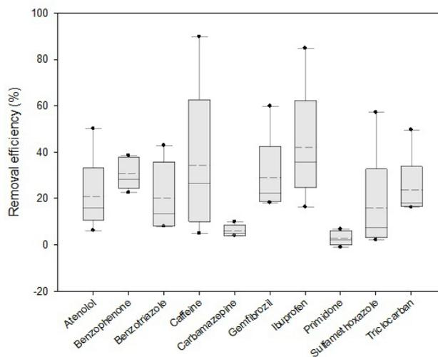
Fig. 3. Removal efficiencies of PPCPs by coagulation treatment at five WRFs (A, B, C, D and E). (Box plot: 25th percentile, median, average and 75th percentile, I: 10th and 90th percentiles.)
