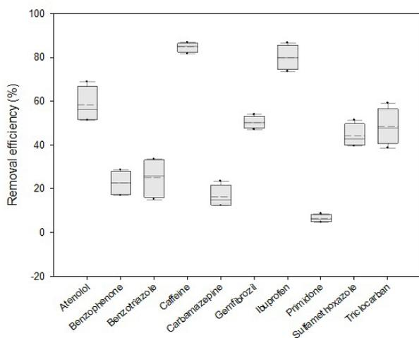
Fig. 2. Removal efficiencies of PPCPs by biological treatment at four WRFs (A, B, C and D). (Box plot: 25th percentile, median, average and 75th percentile, I: 10th and 90th percentiles.)
