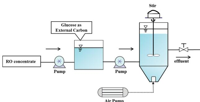
Fig. 1. Schematic diagram of sequencing batch reactor.
