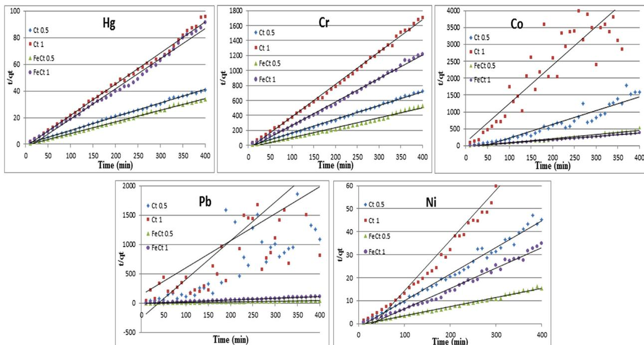
Fig. 5. Pseudo-second-order kinetic adsorption model plots for the adsorption of  $Hg^{2+}$ ,  $Cr^{3+}$ ,  $Co^{2+}$ ,  $Pb^{2+}$ , and  $Ni^{2+}$  ions by two concentrations (0.5 and 1 g) of adsorbents (Ct and FeCt).
