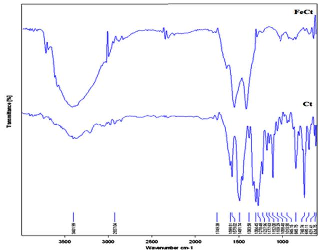
Fig. 1. FTIR of cotton (Ct) and iron nanoparticles impregnated cotton (FeCt).
