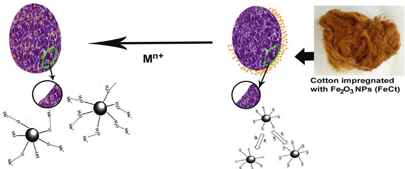
Fig. 7. Schematic depiction of the preparation of FeCt and the adsorption mechanism of heavy metal ions by FeCt.
