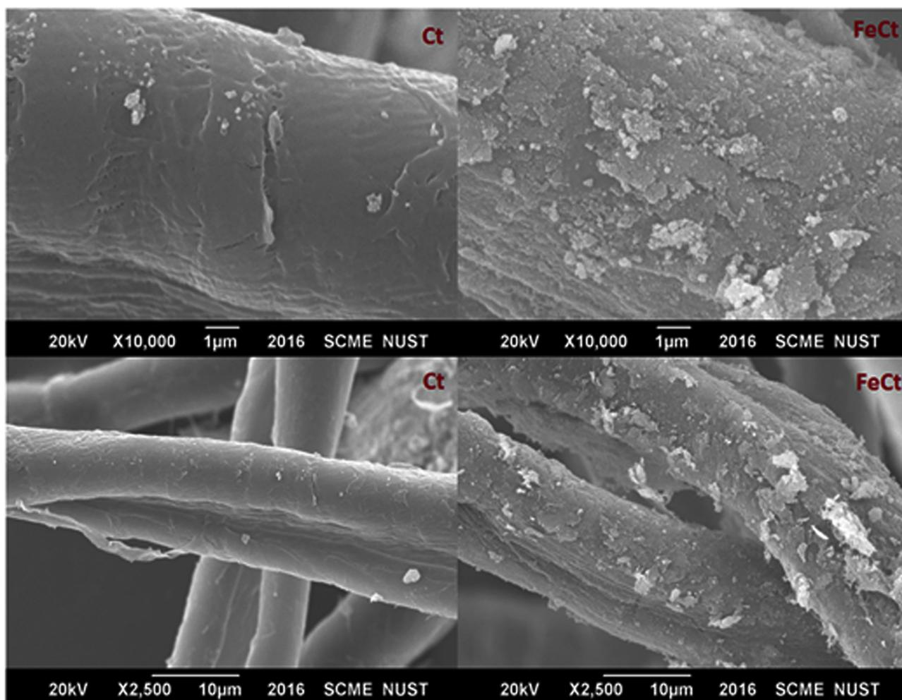
Fig. 3. SEM images of Ct and FeCt nanocomposites.
