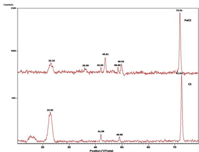
Fig. 2. X-ray diffraction patterns of Ct and FeCt nanocomposites.
