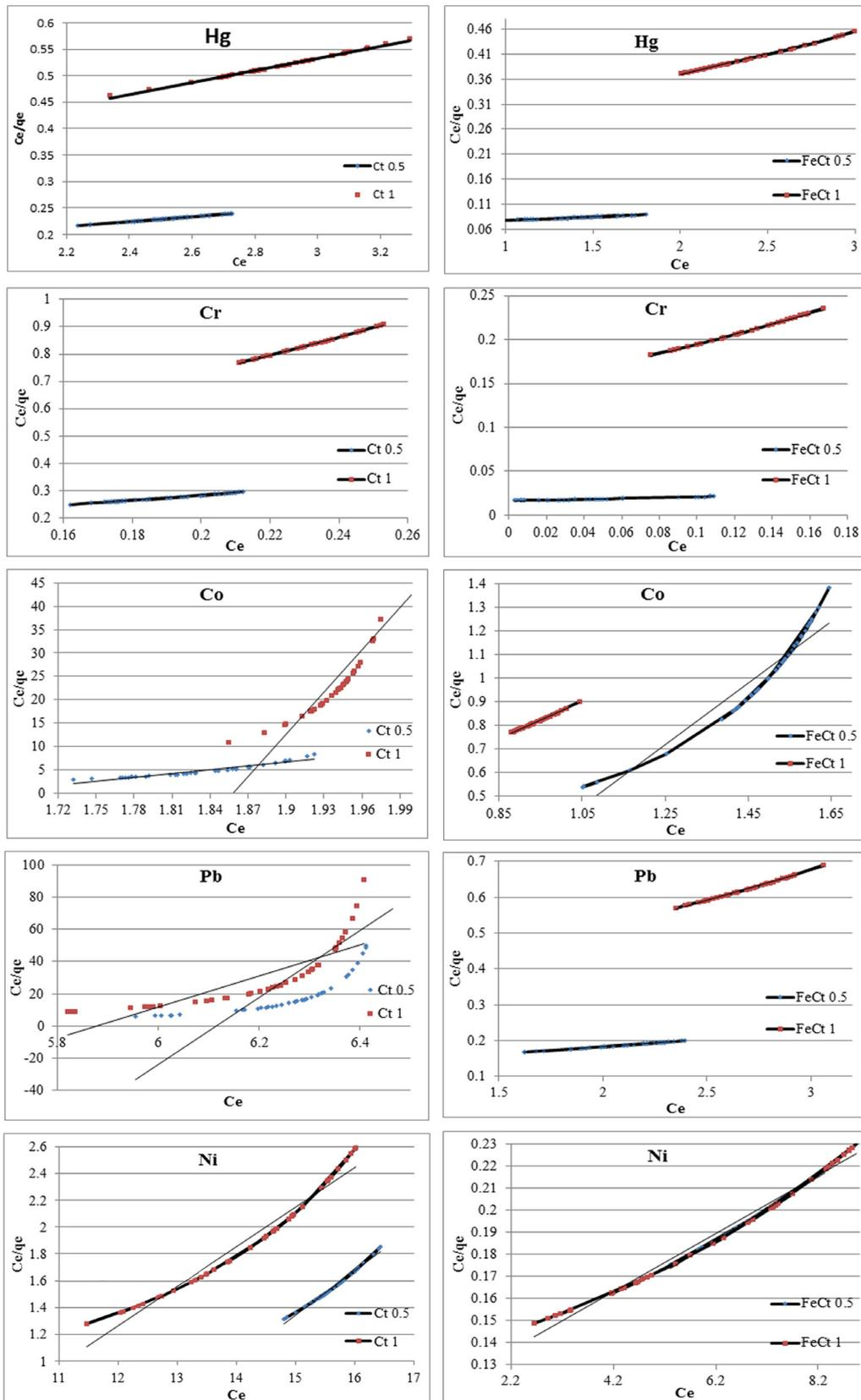
Fig. 6. Adsorption equilibrium isotherm of  $Hg^{2+}$ ,  $Cr^{3+}$ ,  $Co^{2+}$ ,  $Pb^{2+}$ , and  $Ni^{2+}$  removal onto Ct and FeCt at the concentrations of 0.5 and 1 g. Langmuir isotherm fitting curve (equilibrium time 50 min).
