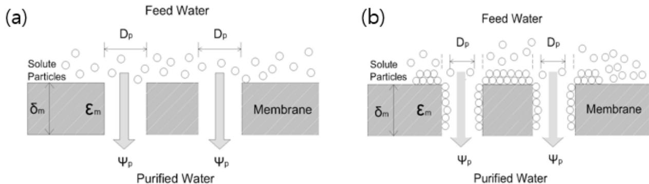
Fig. 1. Particles sticking to membrane surface and pores: (a) virgin state and (b) partly fouled state.
