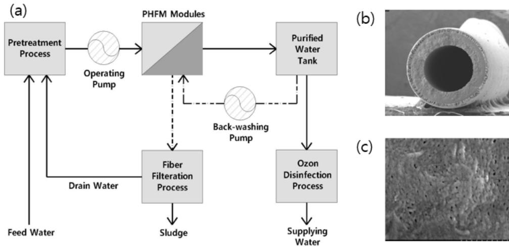
Fig. 3. The membrane system of the plant. (a) Schematic diagram of pressurized PHFM system of the water treatment plant. (b) Photo of cross-section of PHFM. (c) Photo of PHFMs surface.
