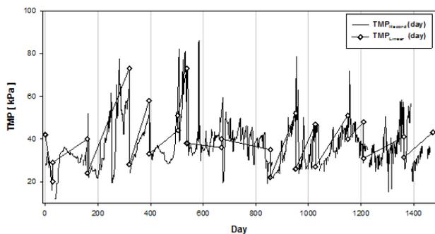
Fig. 4. TMP variation over time during the water treatment.
