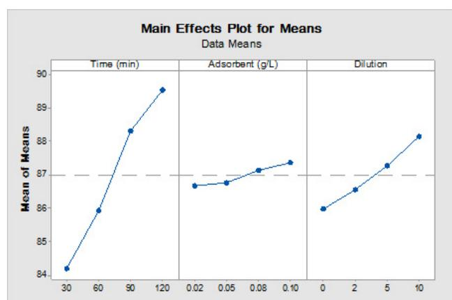
Fig. 4. The main effects plot for means (removal efficiency) of selected parameters (shuffle time, dose of adsorbent and dilution ratio) in removal of nitro-body compounds from spent acid samples by activated carbon particles.
