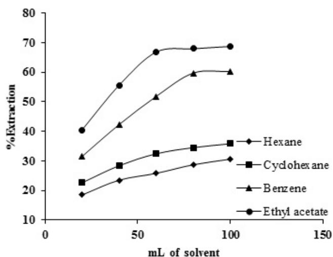
Fig. 1. The effect of solvent on the extraction efficiency of nitro-body compounds from spent acid samples.
