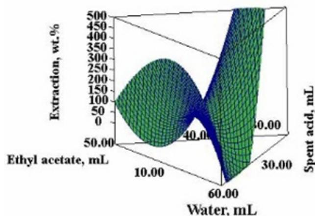
Fig. 3. Response surface plots of water, spent acid and ethyl acetate on the extraction efficiency of nitro-bodies.
