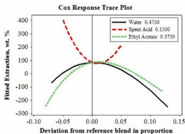
Fig. 2. Response trace plots for the separation of nitro-bodies by ethyl acetate solvent.
