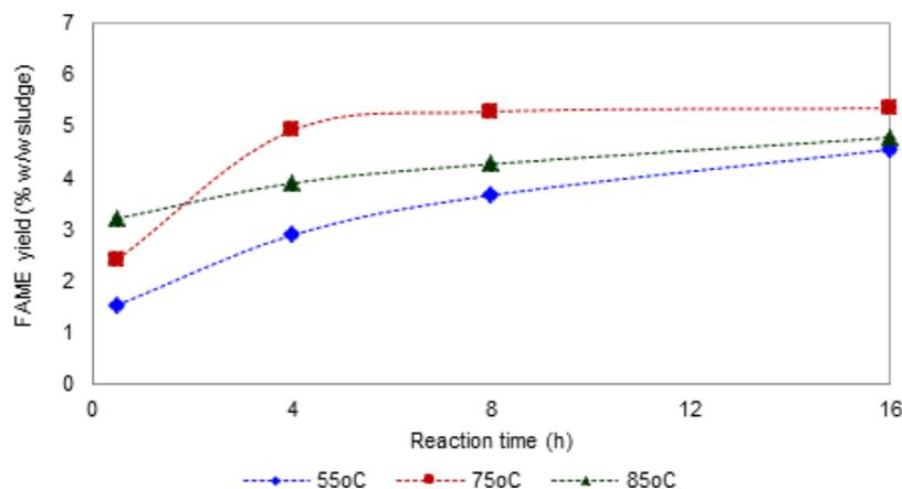
Fig. 3. Effect of reaction temperature under 8:1 methanol to sludge mass ratio and 5% (v/v).
