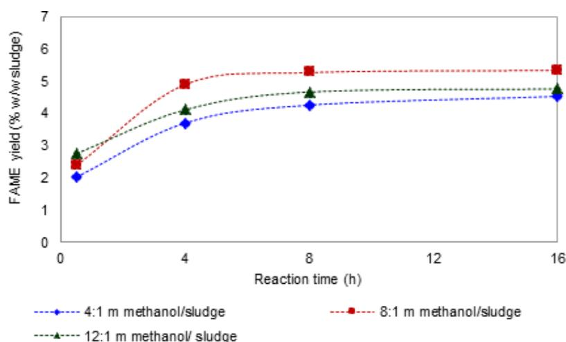
Fig. 1. FAME yield at methanol/sludge mass ratios under 5% (v/v) H<sub>2</sub>SO<sub>4</sub> and 75°C.
