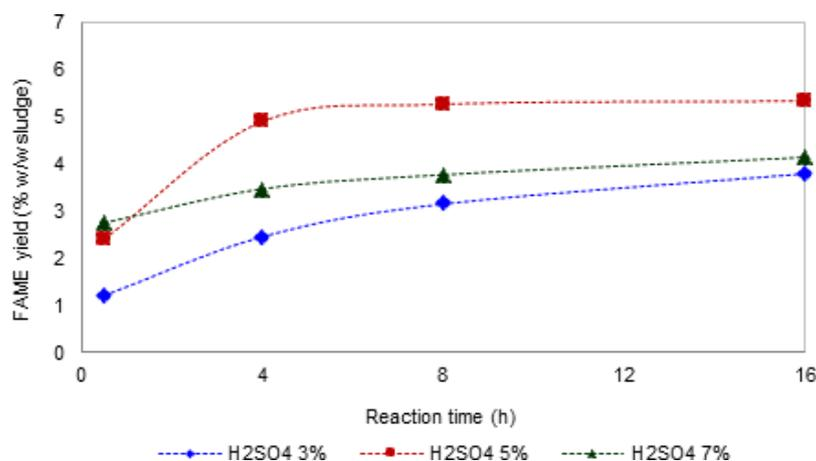
Fig. 2. Effect of  $H_2SO_4$  concentration under 8:1 methanol to sludge mass ratio at 75°C.
