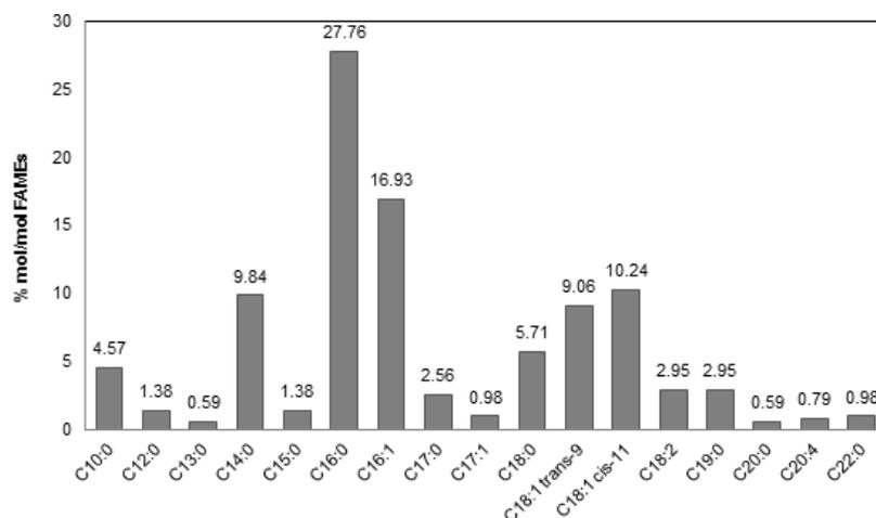
Fig. 4. FAME analysis of biodiesel obtained at 8:1 methanol to sludge mass ratio, 5% (v/v)  $H_2SO_4$ , 75°C and 8 h of reaction time.
