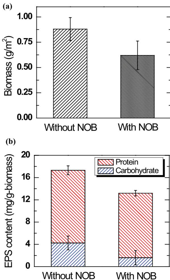
Fig. 4. (a) Mass of biomass and (b) EPS contents of biofilm taken from 25 cm<sup>2</sup> of fouled membranes with and without 5 mg/L of NOB.
