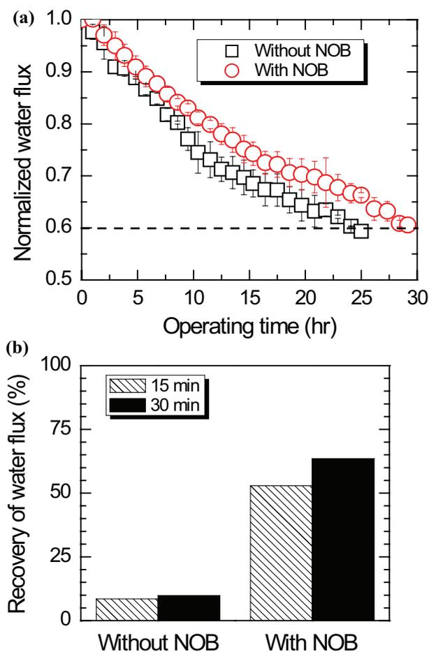
Fig. 1. (a) Change in normalized water flux of both NF membrane systems during accelerated biofouling test and (b) comparison of water flux recovery between two NF membranes after physical cleaning performed for 15 and 30 min.
