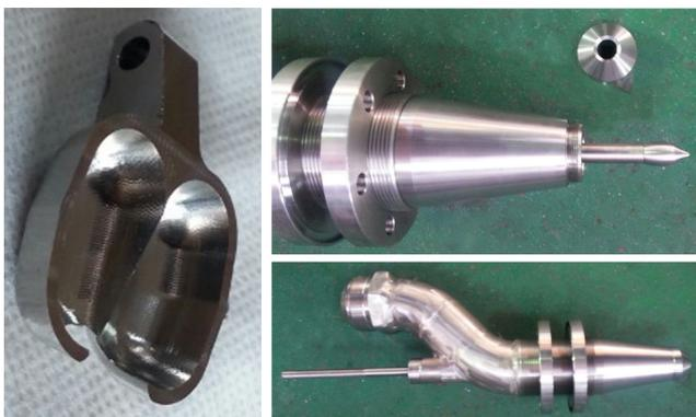
Fig. 5. Manufactured Pelton bucket and spear nozzle.
