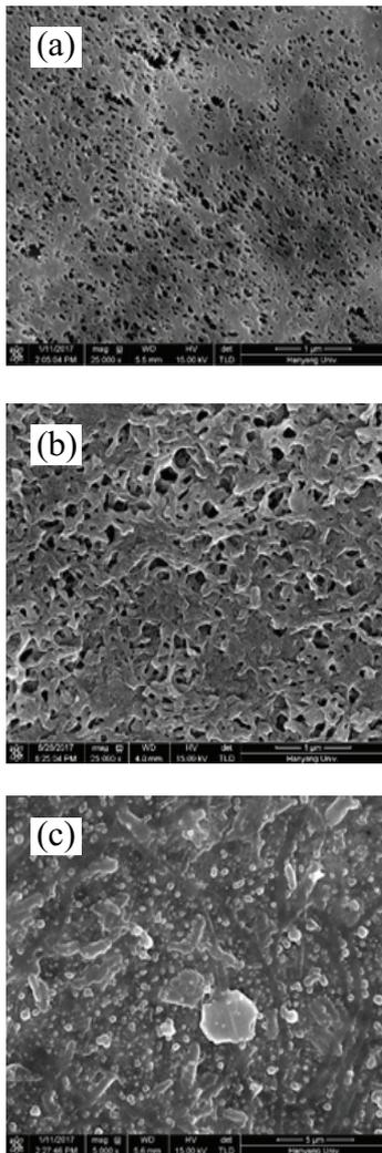
Fig. 3. SEM morphologies of (a) Membrane\_I, (b) Membrane\_LTO and (c) Membrane\_AT.
