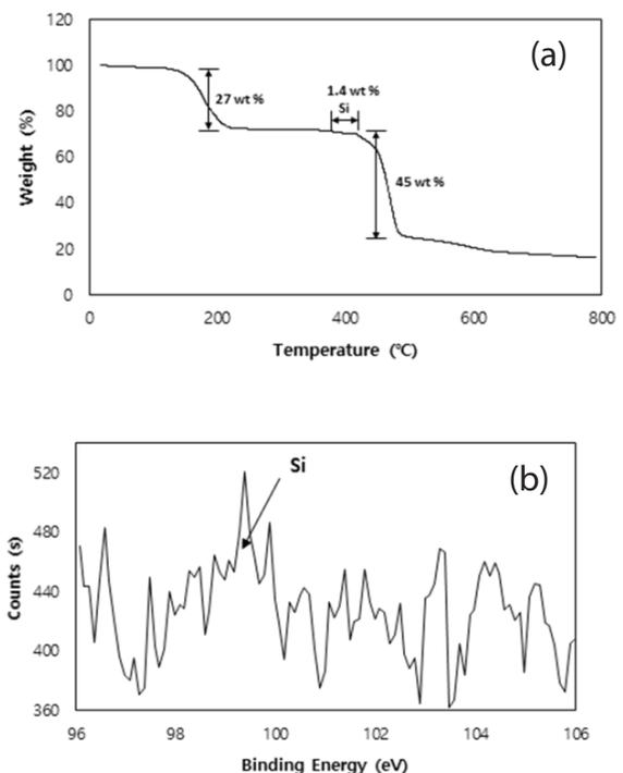
Fig. 2. (a) TGA analysis of Membrane\_I, (b) XPS analysis of Membrane\_I.
