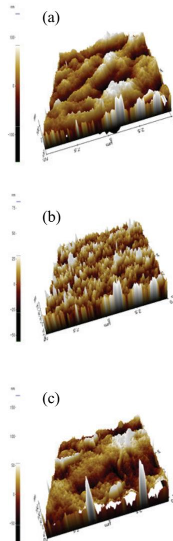
Fig. 4. AFM surface roughness of (a) Membrane\_I, (b) Membrane\_LTO and (c) Membrane\_AT.
