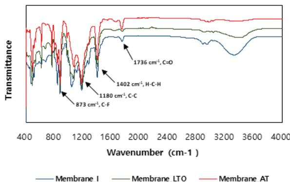
Fig. 1. FT-IR spectra of Membrane\_I, Membrane\_LTO and Membrane\_AT.
