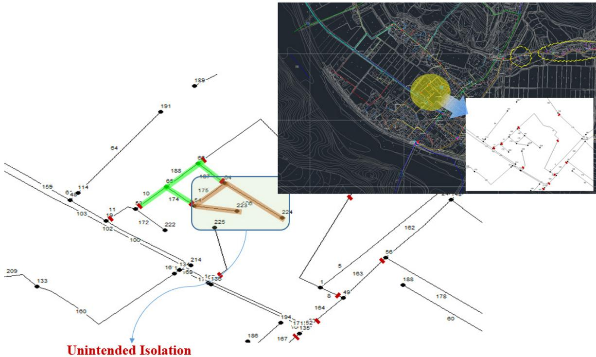
Fig. 7. Sample result of the identified segment and corresponding unintended isolation.
