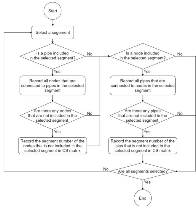
Fig. 4. Algorithms for analyzing the connectivity of segments.
