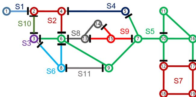
Fig. 3. Identified segments for the sample pipe network.
