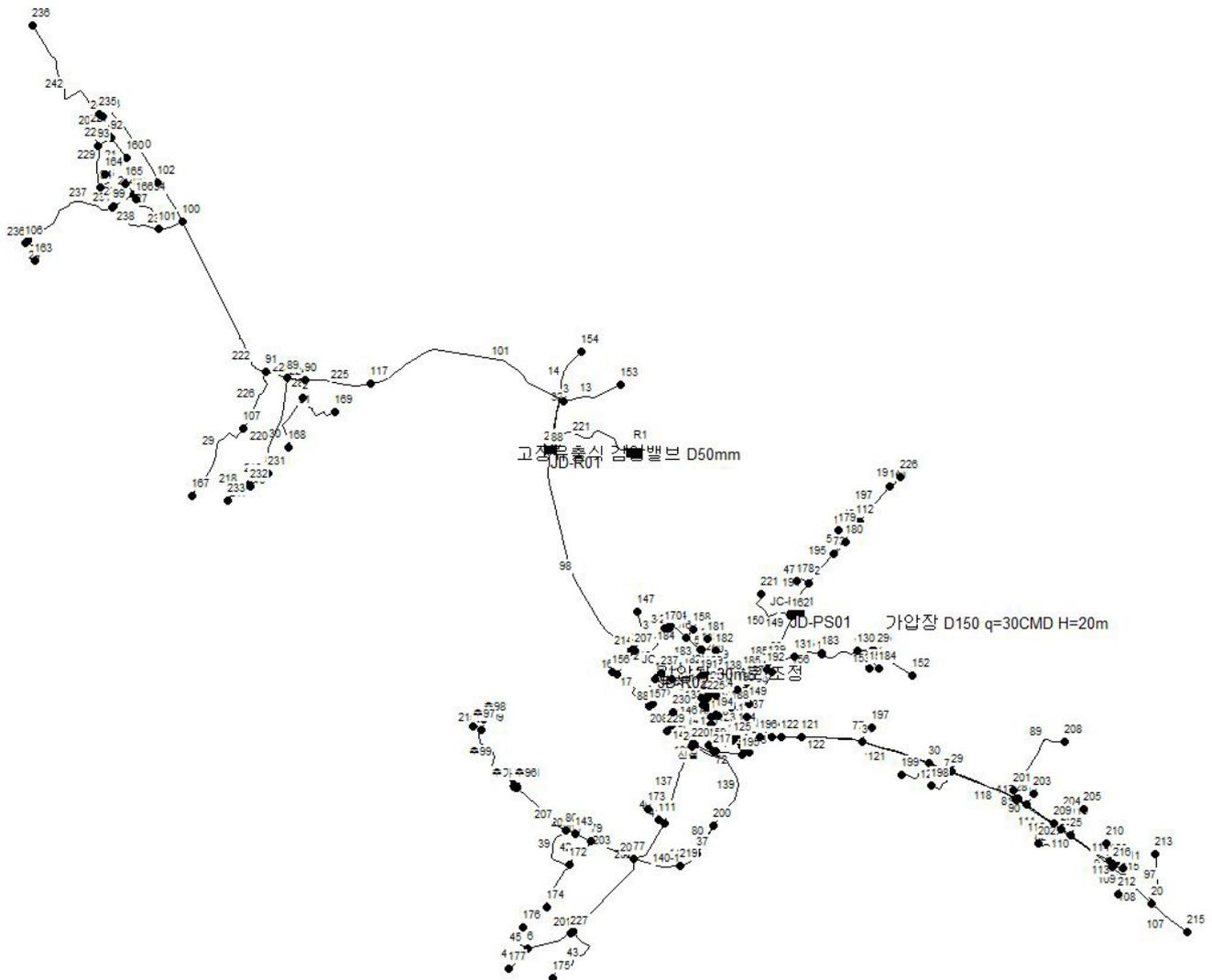
Fig. 6. The pipe network map of the case study water supply system presented by the EPANET program.
