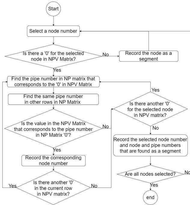
Fig. 1. Algorithm for defining segments in water distribution pipe networks.
