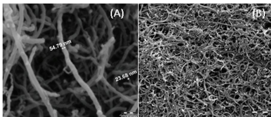
Fig. 2. Size characterization of the MWCNTs at 200 nm magnification (A). (B) The functionalization effect on the MWCNTs after sonication.
