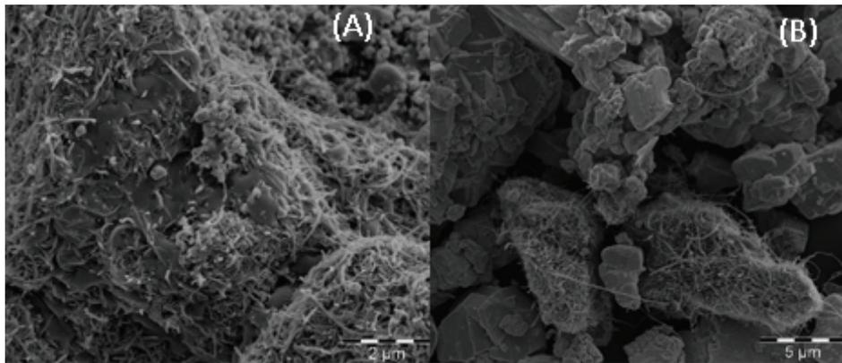
Fig. 3. SEM characterization of (A) silver particles in the presence of the MWCNTs and (B) CuO particles in the presence of MWCNTs.
