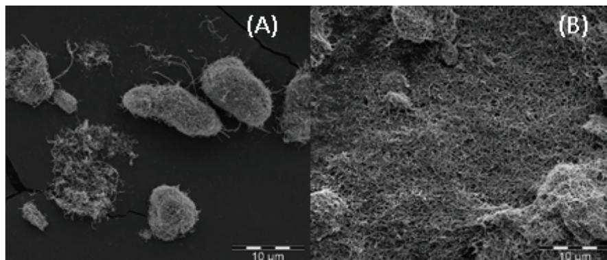
Fig. 1. SEM characterization of MWCNTs. (A) The MWCNTs before treatment exhibited the tendency to agglomerate, decreasing the functionalization capabilities. (B) Effect of 15 min of sonication to separate the nanotubes sufficiently.
