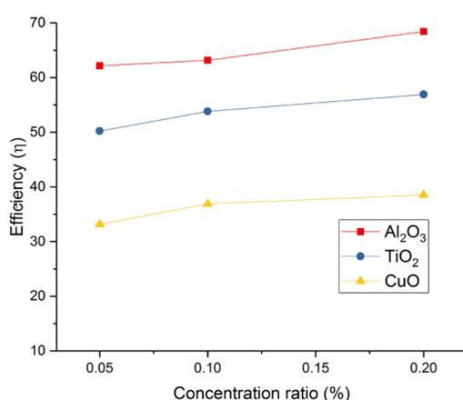
Fig. 6. Variation of daily efficiency of stepped solar still under different concentration of nanofluid.
