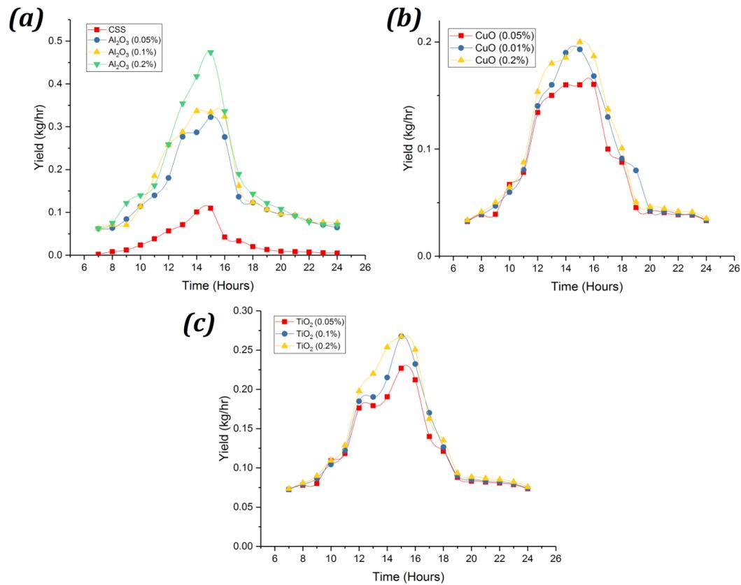
Fig. 4. Hourly variation of yield from stepped solar still with (a) Al<sub>2</sub>O<sub>3</sub>, (b) CuO and (c) TiO<sub>2</sub> nanofluid.
