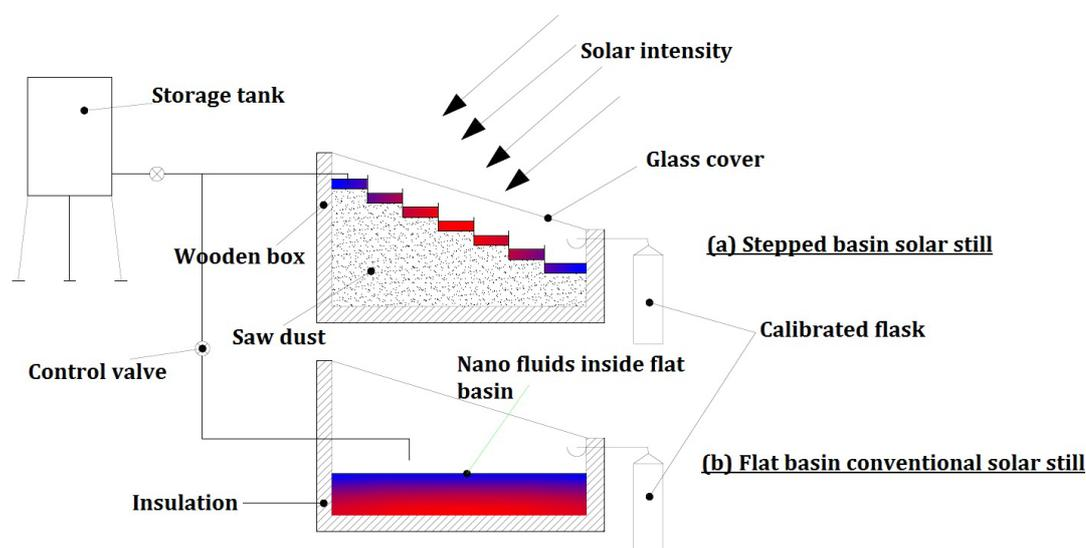
Fig. 1. Schematic diagram of stepped and conventional single slope solar still.
