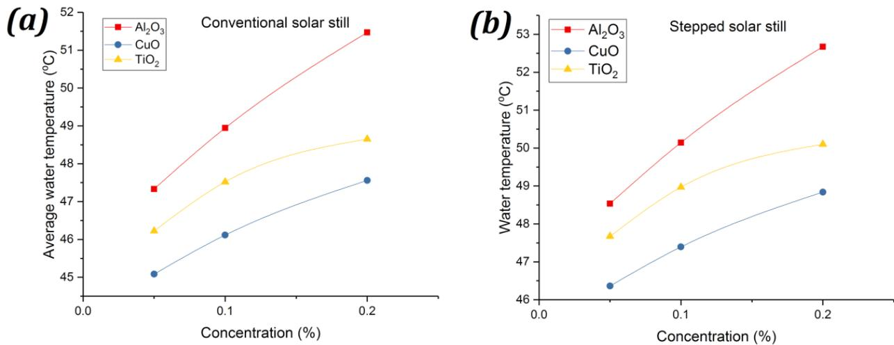
Fig. 5. Variation of average water temperature of (a) Conventional solar still (b) Stepped solar still under different concentration of nanofluid.
