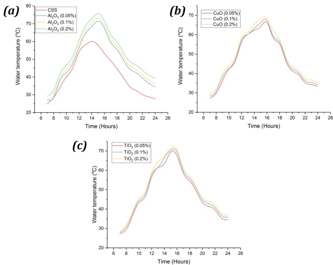
Fig. 3. Hourly variation of water temperature inside stepped solar still with (a) Al<sub>2</sub>O<sub>3</sub>, (b) CuO and (c) TiO<sub>2</sub> nanofluid.
