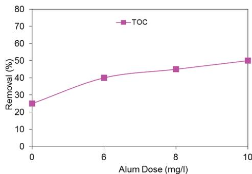
Fig. 5. Effect of coagulant dose on MF performance in terms of TOC removal.
