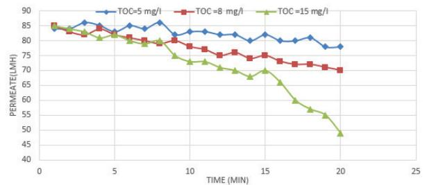
Fig. 3. Effect of initial TOC concentration on the permeate flux of MF membrane.
