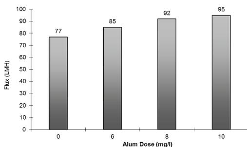
Fig. 6. Effect of coagulant dose on the MF permeate flux.
