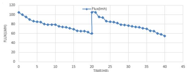
Fig. 4. Permeate flux after hydraulic backwashing and chemical cleaning.
