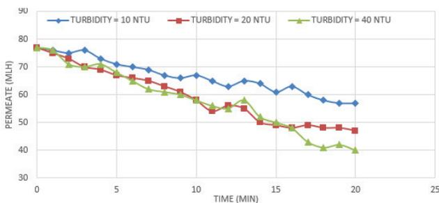
Fig. 2. Effect of initial turbidity on the MF membrane performance in terms of permeate flux.
