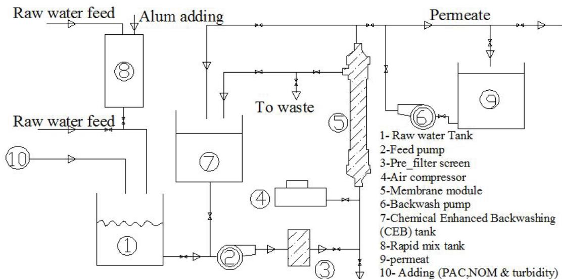
Fig. 1. Process flow diagram of the PALL microfiltration pilot plant.
