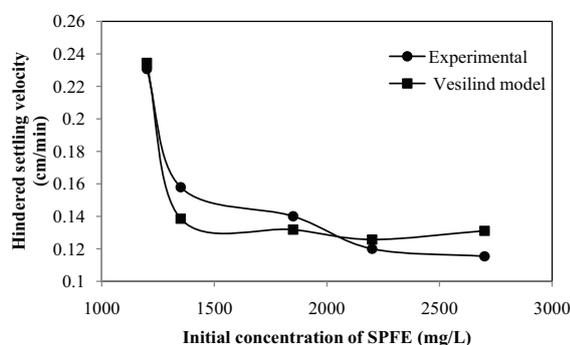
Fig. 21. Settling velocity as a function of the solids concentration.
