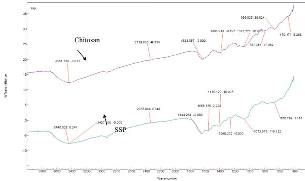
Fig. 5. FTIR spectrum of SSP and chitosan.
