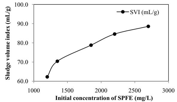
Fig. 19. Sludge volume index as a function of the initial concentration.
