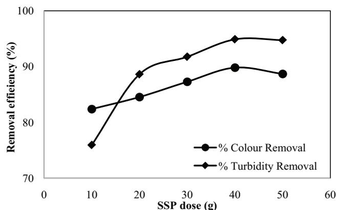
Fig. 10. Impact of coagulant SSP dose on removal efficiency. SPFE volume: 1 L; initial pH of SPFE (actual): 8.4–8.6; initial concentration of SPFE: 1,200 mg/L; coagulant: extragens = 10–50 g of SSP: 3 N NaCl; coagulant-eluate volume: 1 L.
