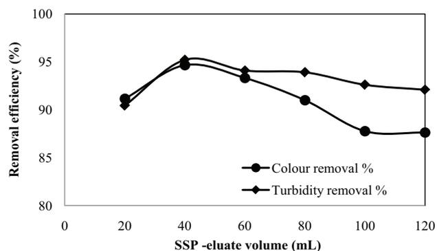
Fig. 11. Impact of coagulant SSP-eluate volume on removal efficiency. SPFE volume: 1 L; initial pH of SPFE (actual): 8.4–8.6; initial concentration of SPFE: 1,200 mg/L; coagulant: extragens = 40 g of SSP: 3 N NaCl; coagulant-eluate volume: 200–1,200 mL.
