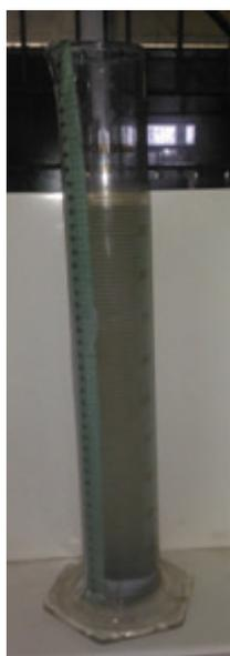
Fig. 4. Photograph of the batch settling column.
