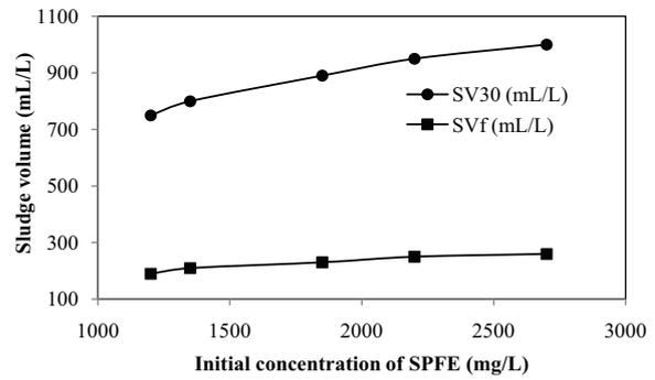
Fig. 18. Sludge volume as a function of the initial concentration.
