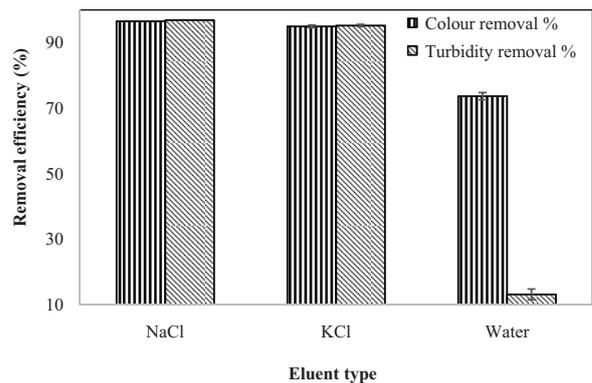
Fig. 8. Impact of eluent type on removal efficiency. SPFE volume: 1 L; initial pH of SPFE (actual): 8.4–8.6; initial concentration of SPFE: 1,200 mg/L; coagulant: extragens = 30 g of SSP: 3 N NaCl, 3 N KCl, distilled water; coagulant-eluate volume: 1 L.
