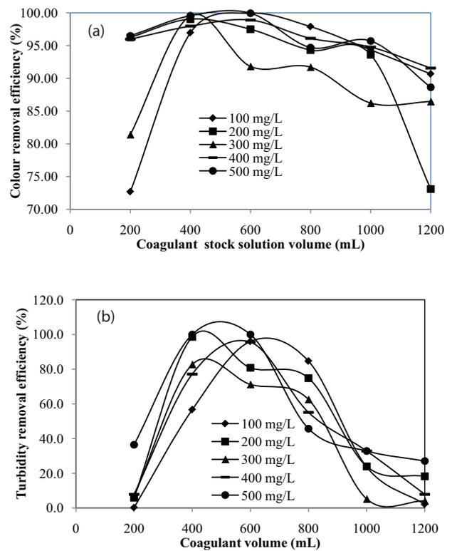
Fig. 15. (a) Impact of chitosan volume on colour removal efficiency. (b) Impact of chitosan volume on turbidity removal efficiency. SPFE volume: 1 L; initial pH of SPFE (actual): 8.4–8.6; initial concentration of SPFE: 1,200 mg/L.
