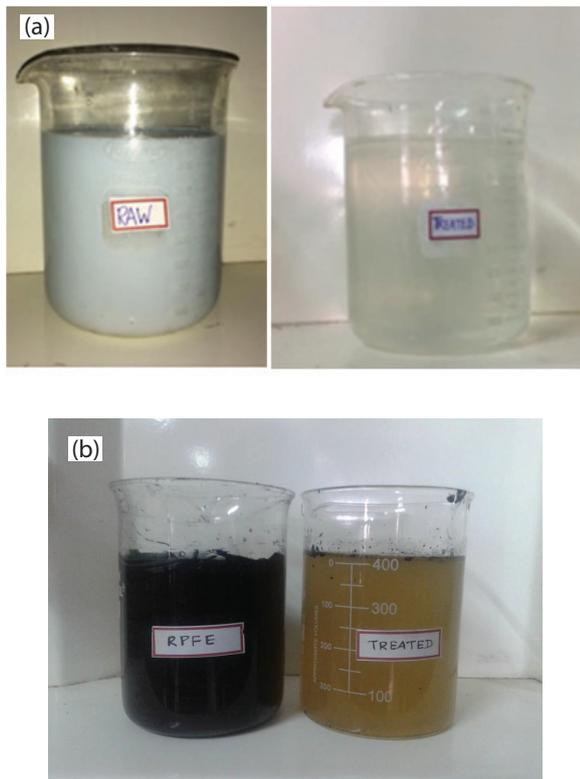
Fig. 14. Photographs of (a) SPFE and (b) RPFE before and after treatment using SSP.
