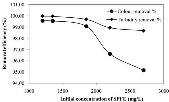
Fig. 17. Impact of initial concentration of SPFE on removal efficiency. SPFE volume: 1 L; chitosan concentration: 500 mg/L; chitosan stock solution volume: 600 mL; initial pH of SPFE (actual): 8.4–8.6.
