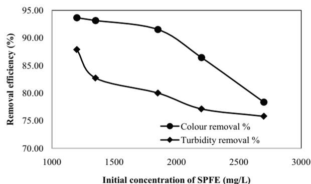
Fig. 13. Impact of initial concentration of SPFE on removal efficiency. SPFE volume: 1 L; initial pH of SPFE (actual): 8.2–8.6; initial concentration of SPFE: 1,200–2,700 mg/L; coagulant: extragens = 40 g of SSP: 3 N NaCl; coagulant-eluate volume: 400 mL.
