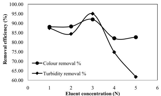
Fig. 9. Impact of eluent concentration on removal efficiency. SPFE volume: 1 L; initial pH of SPFE (actual): 8.4–8.6; initial concentration of SPFE: 1,200 mg/L; coagulant: extragens = 30 g of SSP: NaCl (1–5 N); coagulant-eluate volume: 1 L.
