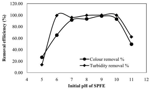
Fig. 16. Impact of initial pH of SPFE on removal efficiency. SPFE volume: 1 L; chitosan concentration: 500 mg/L; chitosan stock solution volume: 600 mL; initial concentration of SPFE: 1,200 mg/L.
