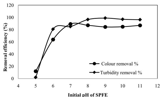
Fig. 12. Impact of initial pH of SPFE on removal efficiency. SPFE volume: 1 L; initial pH of SPFE: 5–11; initial concentration of SPFE: 1,200 mg/L; coagulant: extragens = 40 g of SSP: 3 N NaCl; coagulant-eluate volume: 400 mL.
