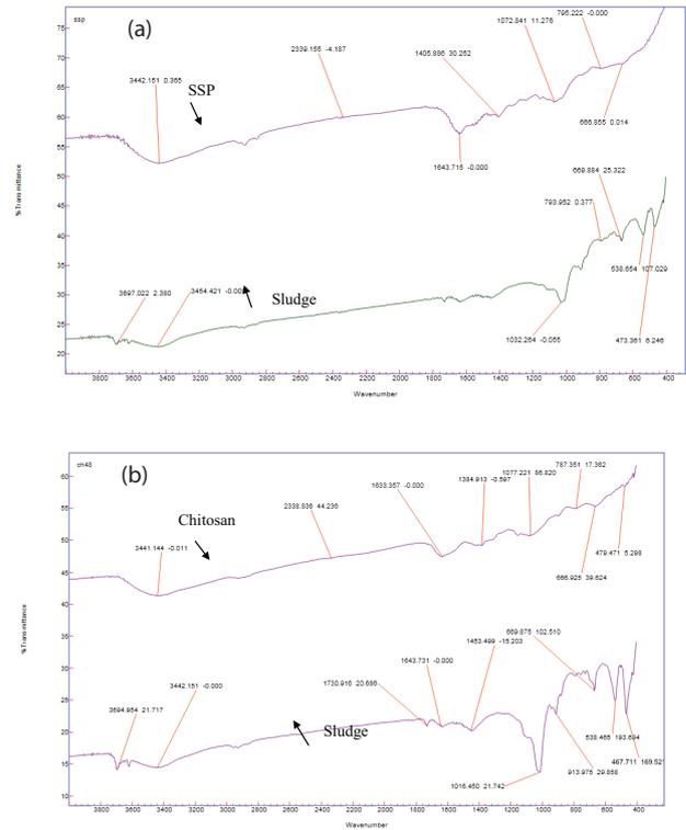
Fig. 6. (a) FTIR spectrum of SSP and sludge treated using SSP. (b) FTIR spectrum of chitosan and sludge treated using chitosan.
