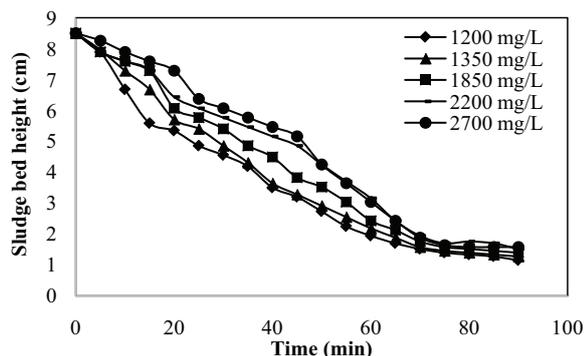
Fig. 20. Batch settling curves at different initial concentrations.
