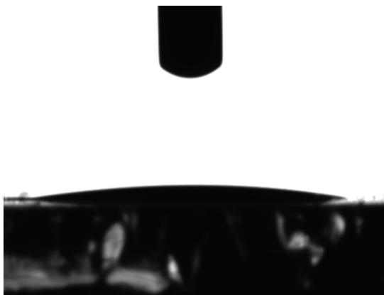
Fig. 5. Contact angle of water on ZnO nanostructured film.
