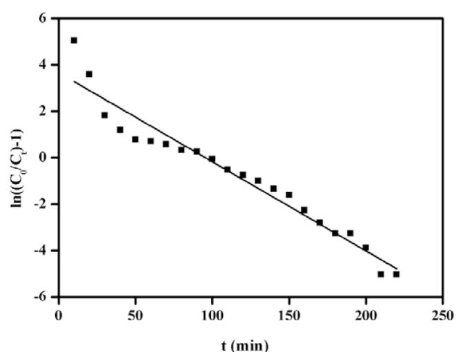
Fig. 12. Plot of  $\ln((C_0/C_t)-1)$  vs.  $t$  according to Thomas model.
