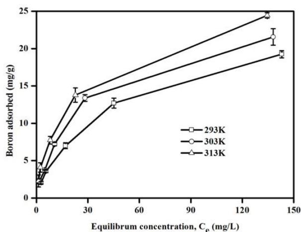
Fig. 8. Adsorption isotherms of boron onto LSC-800 resin at different temperatures. Boron concentration = 5–200 mg/L, resin dosage = 4 g/L, pH = 9, contact time = 2 h.
