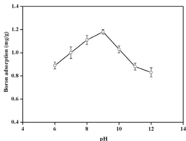
Fig. 4. Effect of initial pH on boron removal by LSC-800 resin. Boron concentration = 5 mg/L, resin dosage = 4 g/L,  $T = 30^{\circ}\text{C}$ , contact time = 2 h.
