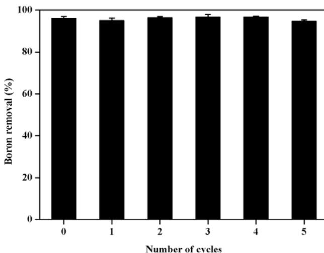
Fig. 10. Boron removal capacity of the regenerated resin. Feed boron concentration = 5 mg/L, resin dosage = 4 g/L, pH = 9, T = 30 °C.
