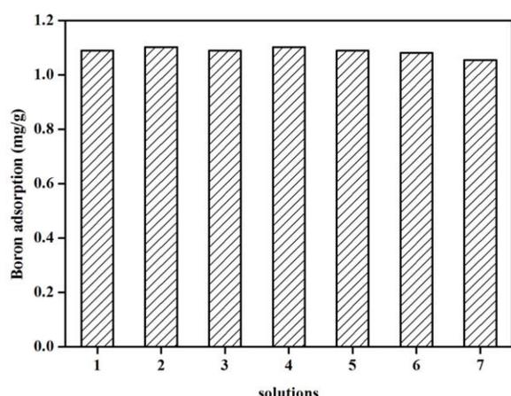
Fig. 7. Effect of foreign ions on boron removal by LSC-800 resin at pH 9 ((1) 5 mg B/L  $H_3BO_3$ ; (2) 5 mg B/L  $H_3BO_3$  + 0.01 mol/L NaCl; (3) 5 mg B/L  $H_3BO_3$  + 0.1 mol/L NaCl; (4) 5 mg B/L  $H_3BO_3$  + 0.01 mol/L  $CaCl_2$ ; (5) 5 mg B/L  $H_3BO_3$  + 0.1 mol/L  $CaCl_2$ ; (6) 5 mg B/L  $H_3BO_3$  + 0.01 mol/L  $MgSO_4$ ; (7) 5 mg B/L  $H_3BO_3$  + 0.1 mol/L  $MgSO_4$ ).
