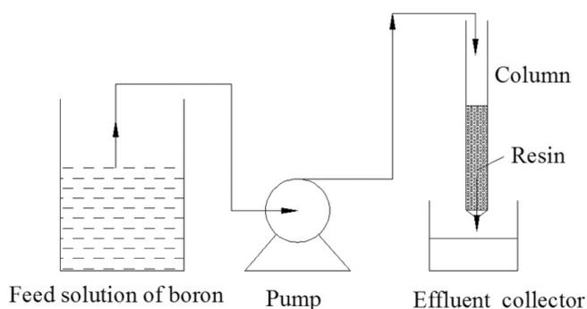
Fig. 1. Schematic diagram of experimental set-up for column adsorption.
