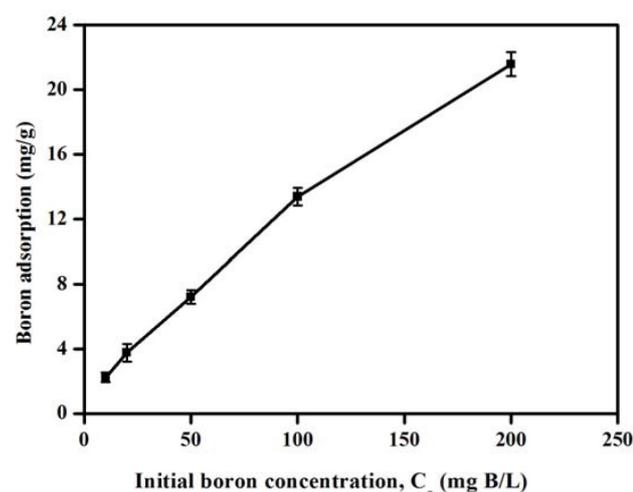
Fig. 6. Effect of initial boron concentration on boron removal by LSC-800 resin. Resin dosage = 4 g/L,  $\text{pH} = 9$ ,  $T = 30^{\circ}\text{C}$ , contact time = 2 h.
