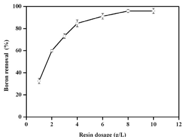
Fig. 5. Effect of resin dosage on boron removal by LSC-800 resin. Boron concentration = 5 mg/L,  $\text{pH} = 9$ ,  $T = 30^{\circ}\text{C}$ , contact time = 2 h.
