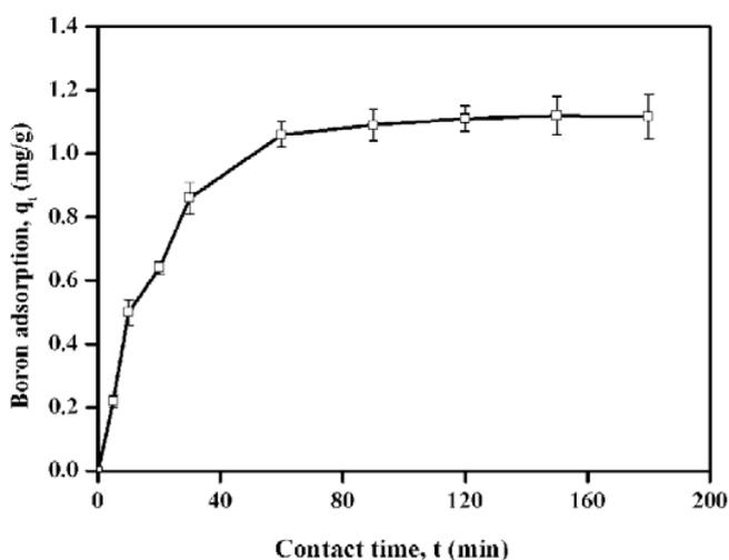
Fig. 2. Effect of contact time on boron removal by LSC-800 resin. Boron concentration = 5 mg/L, resin dosage = 4 g/L, pH = 9, T = 30°C.
