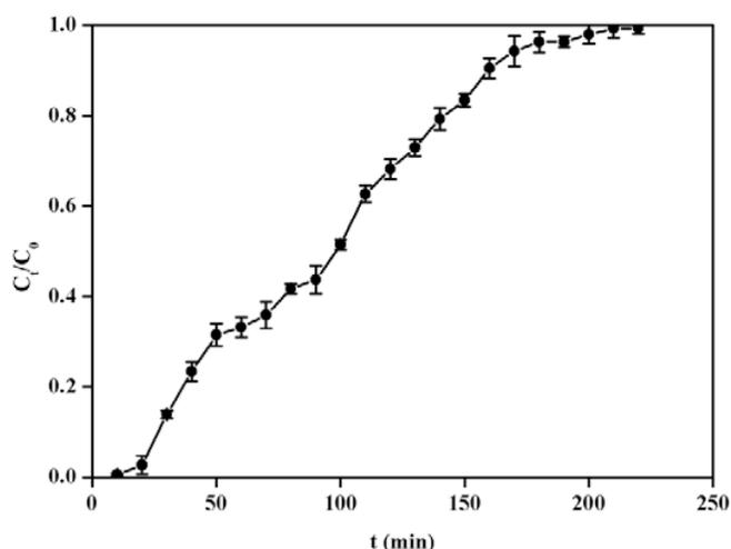
Fig. 11. Breakthrough curve of boron adsorption onto LSC-800 resin.
