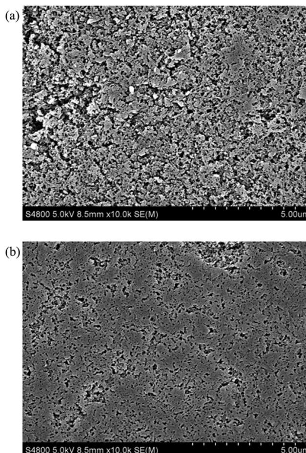
Fig. 3. SEM micrographs of LSC-800 resin (a) before and (b) after adsorption of boron.
