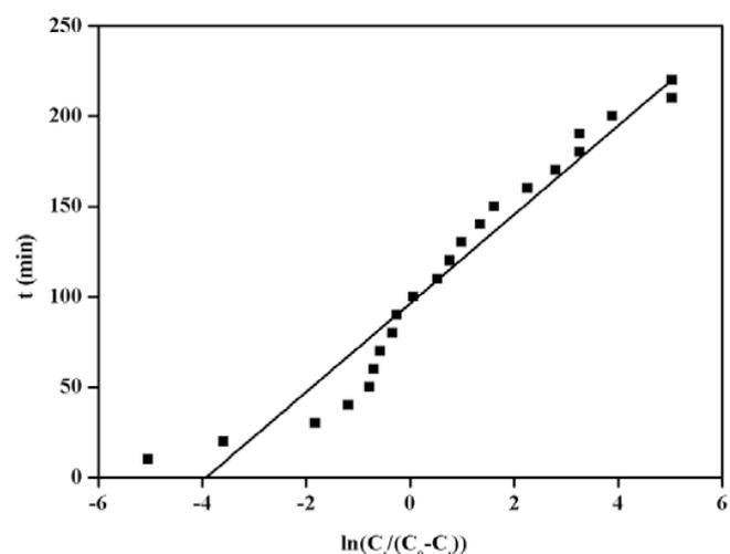
Fig. 13. Plot of  $\ln(C_t/(C_0 - C_t))$  vs.  $t$  according to Yoon and Nelson model.
