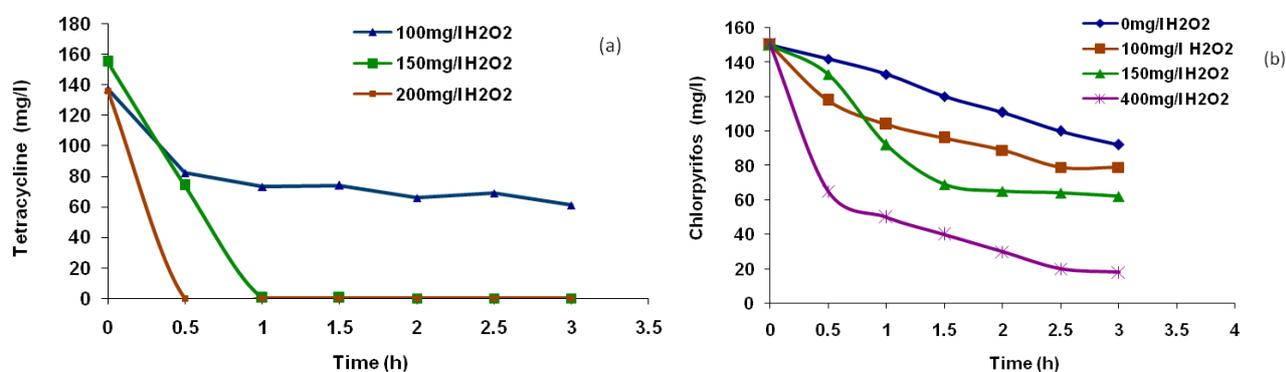
Fig. 4. Variation of tetracycline (a) and chlorpyrifos (b) conc. in wastewater against illumination time at different concentration of  $\text{H}_2\text{O}_2$  (pH = 3,  $\text{Fe}^{2+}$  = 50 mg/l,  $\text{TiO}_2$  = 100 mg/l).
