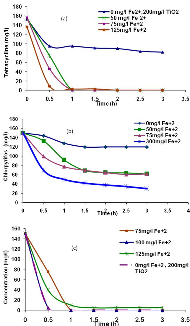
Fig. 7. Variation of tetracycline (a), chlorpyrifos (b) and xylene (c) concentrations in wastewater against illumination time at different concentration of  $\text{Fe}^{2+}$  ( $\text{pH} = 3$ ,  $\text{TiO}_2 = 100 \text{ mg/l}$ ,  $\text{H}_2\text{O}_2 = 200 \text{ mg/l}$ ).
