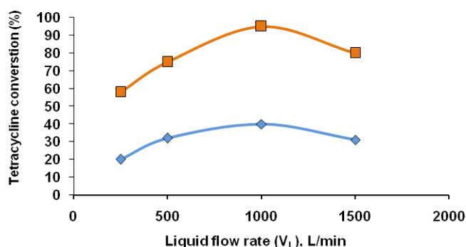
Fig. 8. Variation of tetracycline conversion in wastewater against liquid flow rate at different concentration of  $\text{TiO}_2$  (■:  $\text{CTiO}_2 = 100 \text{ mg/L}$ ; ♦:  $\text{CTiO}_2 = 0 \text{ mg/L}$ ), ( $\text{pH} = 3$ ,  $\text{Fe}^{2+} = 125 \text{ mg/L}$ ,  $\text{H}_2\text{O}_2 = 200 \text{ mg/L}$ ).
