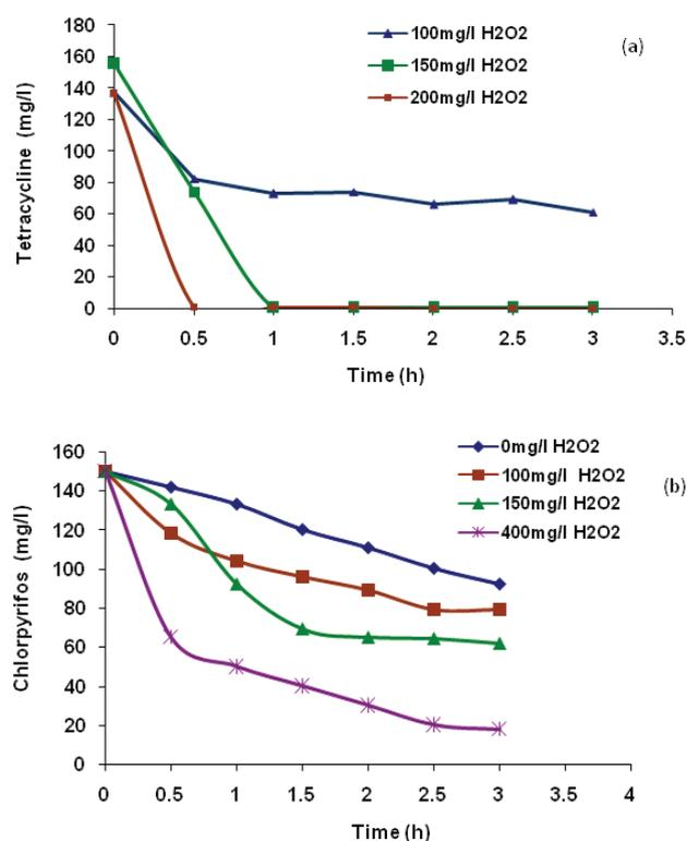
Fig. 5. Variation of tetracycline (a) and chlorpyrifos (b) conc. in wastewater against illumination time at different concentration of TiO<sub>2</sub> (pH = 3, Fe<sup>2+</sup> = 125 mg/L, H<sub>2</sub>O<sub>2</sub> = 200 mg/L).
