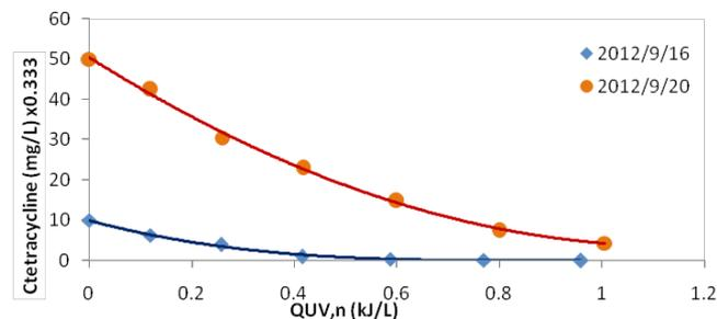
Fig. 6. Variation of tetracycline concentration in wastewater against illumination time at different concentration of tetracycline (pH = 3, Fe<sup>2+</sup> = 125 mg/L, TiO<sub>2</sub> = 50 mg/L, H<sub>2</sub>O<sub>2</sub> = 150 mg/L).
