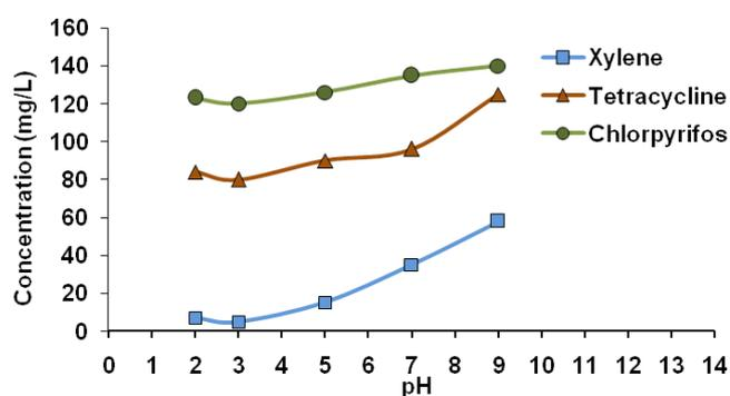
Fig. 3. Relationship between pH and concentration after 30 min at ( $H_2O_2$  150 mg/L,  $TiO_2$  100 mg/L,  $Fe^{+2}$  50 mg/L).
