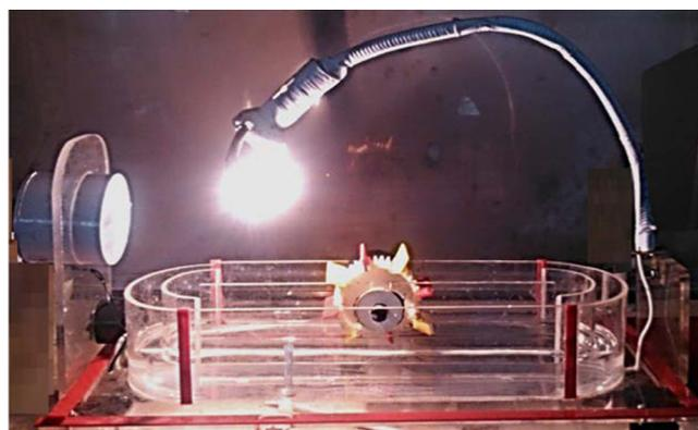
Fig. 1. Experimental set-up of the fiberglass-Raceway Pond Reactor (RPR) with a maximum capacity of 7.5 L.
