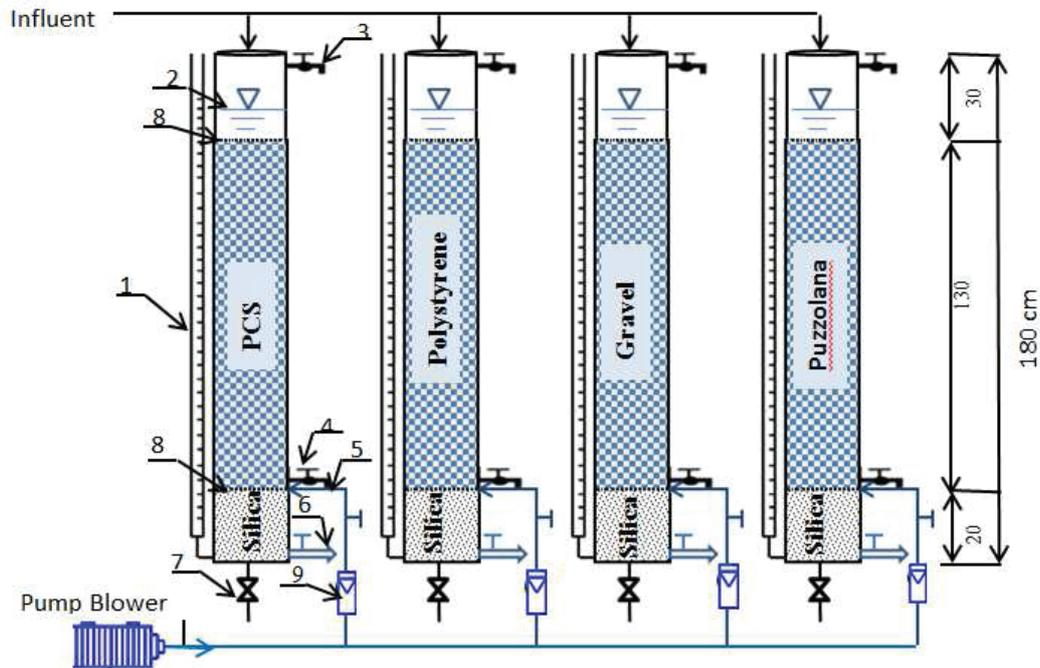
Fig. 2. Schematic diagram of BAFs' configuration system. (1) Piezometer (water level indicator); (2) Water level; (3) Top backwashing valve; (4) Bottom backwashing valve; (5) Air inlet; (6) Effluent; (7) Air and water backwashing inlet; (8) Stainless steel net; (9) Air flow meter.
