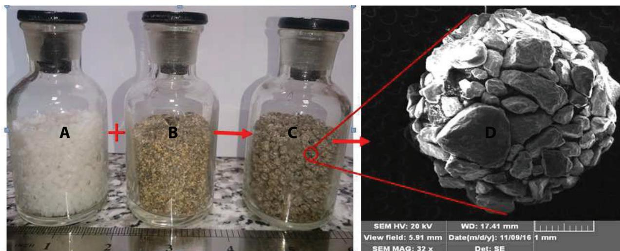
Fig. 1. Production diagram of PCS media. A: crystal granules of HIPS7240 polystyrene, B: sand particles, C: PCS media and D: SEM of PCS media.
