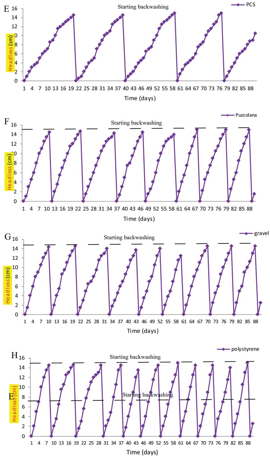
Fig. 4. Comparison of hydraulic head loss and back washing at the BAFs during the backwash intervals. E: PCS; F: Puzzolana; G: Gravel; H: Polystyrene.
