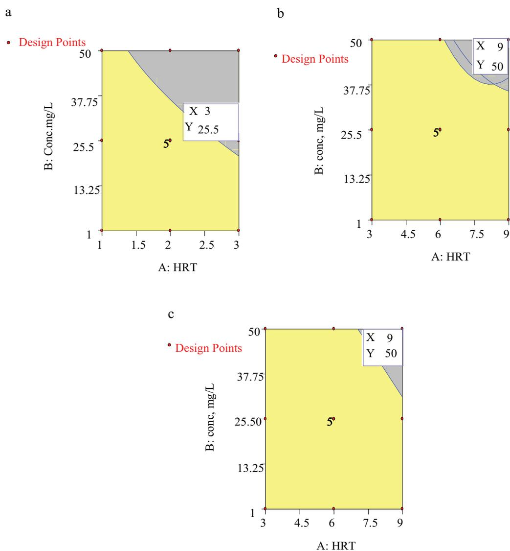
Fig. 4. Overlay plot for optimal region for removal pollutants from a) anaerobic stabilization pond, b) facultative stabilization pond and c) maturation stabilization pond.
