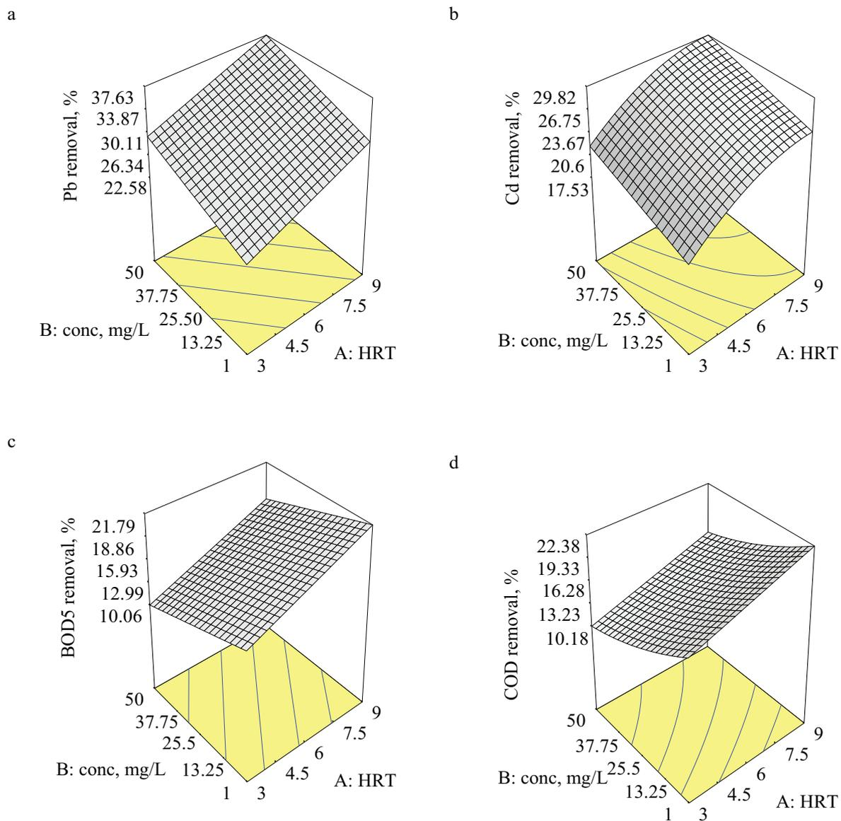
Fig 3. Response surface plot for maturation stabilization pond (a) Pb removal (b) Cd removal (c) BOD5 removal and (d) COD removal.
