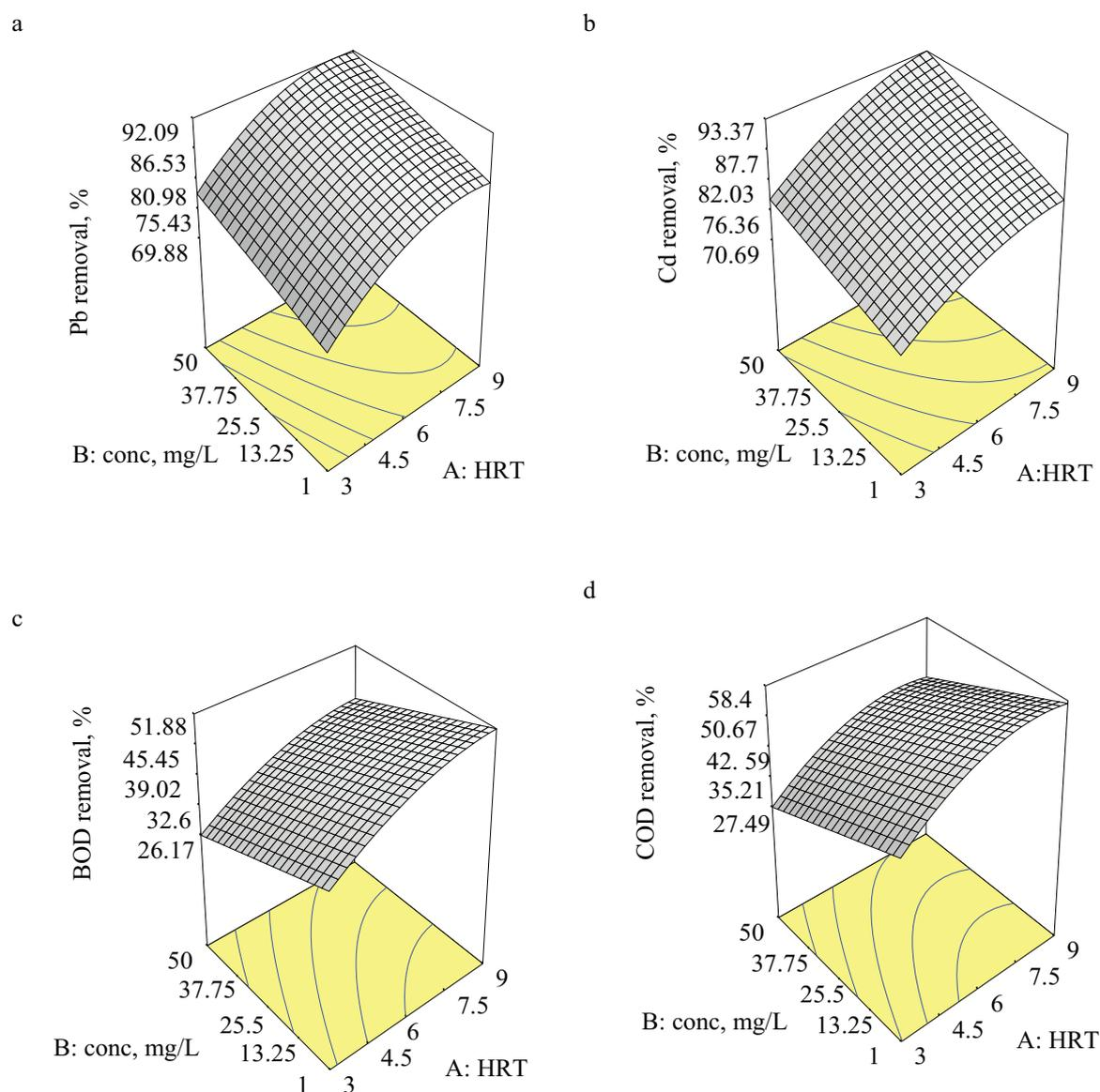
Fig. 2. Response surface plot for facultative stabilization pond (a) Pb removal (b) Cd removal (c) BOD<sub>5</sub> removal and (d) COD removal.
