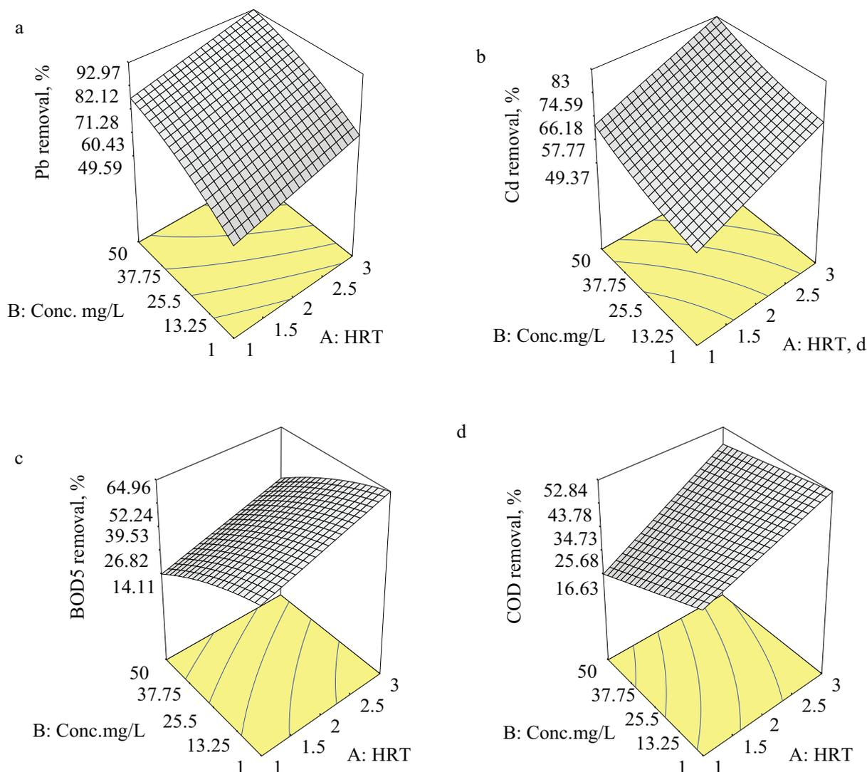
Fig. 1. Response surface plot for anaerobic stabilization pond (a) Pb removal (b) Cd removal (c) BOD5 removal and (d) COD removal.
