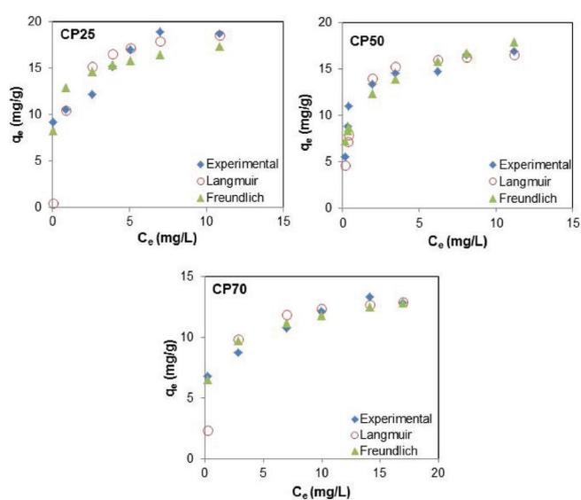
Fig. 5. Experimental and theoretical Cu(II) adsorption isotherms ( $C_0 = 20$  mg/L, adsorbent concentration: 2 g/L, pH = 5.6, T = 25°C, contact time = 75 min).
