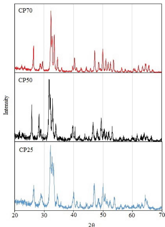
Fig. 1. X-ray diffraction patterns of calcium phosphate powders.
