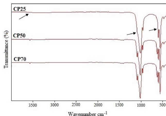
Fig. 2. FT-IR spectrums of calcium phosphate powders.
