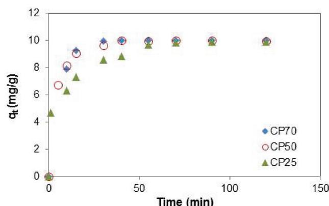
Fig. 6. Effect of contact time on the adsorption ( $C_0 = 20$  mg/L, adsorbent concentration: 2 g/L, pH = 5.6,  $T = 25^\circ\text{C}$ ).
