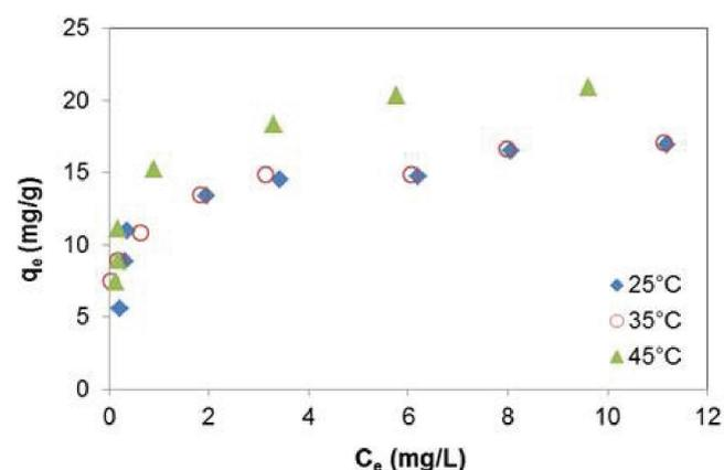
Fig. 4. Experimental Cu(II) adsorption isotherms of CP50 at different temperatures ( $C_0 = 20$  mg/L, adsorbent concentration: 2 g/L, pH = 5.6, contact time = 75 min).
