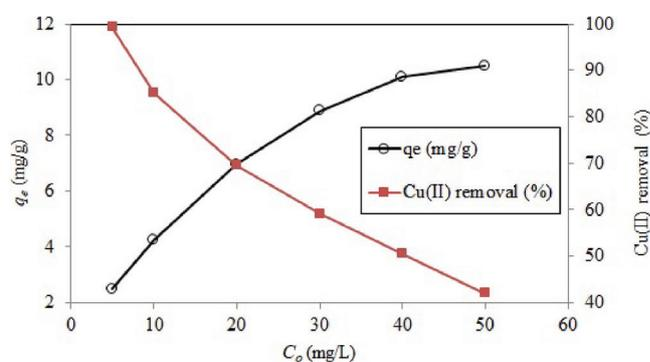
Fig. 3. Effect of initial Cu(II) concentration on adsorption (adsorbent (CP70) concentration: 2 g/L, pH = 5.6, T = 25°C, contact time = 120 min).
