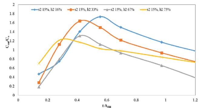
Fig. 15. Time of maximum concentration for different outlet baffle vertical positions (h2 = 16%, 33%, 65% and 75; and s2 = 15% of the length).
