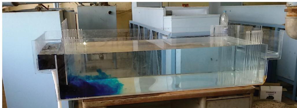
Fig. 1. Photo of the pilot scale sedimentation tank.
