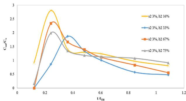
Fig. 11. Time of maximum concentration for different outlet baffle vertical locations (h2 = 16%, 33%, 65% and 75; and s2 = 3% of the length).
