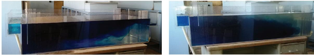
Fig. 7. Photo of dye evolution for the cases that baffle is located at h1: 33% and s1: 3% (left photo) and h1: 67% and s1: 5% (right photo).
