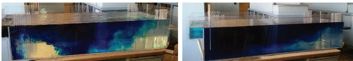
Fig. 4. Photos of dye evolution in without inlet baffle case (left) and with inlet baffle located at h1: 33% and s1: 3% (right).
