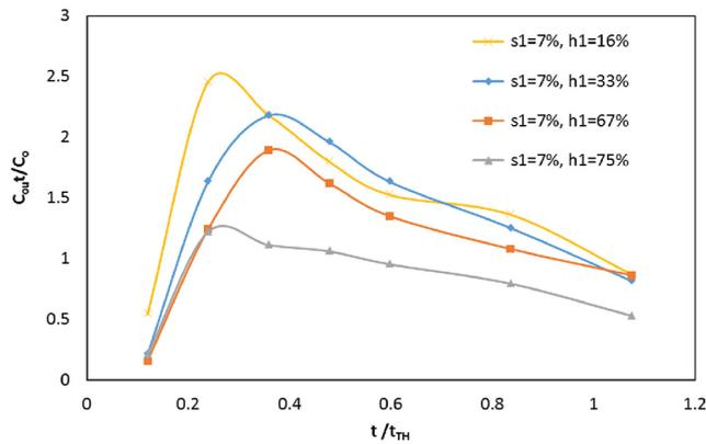
Fig. 8. Time of maximum concentration for different inlet baffle vertical positions (h1 = 16%, 33%, 65%, 75%; and s1 = 7% of the length).
