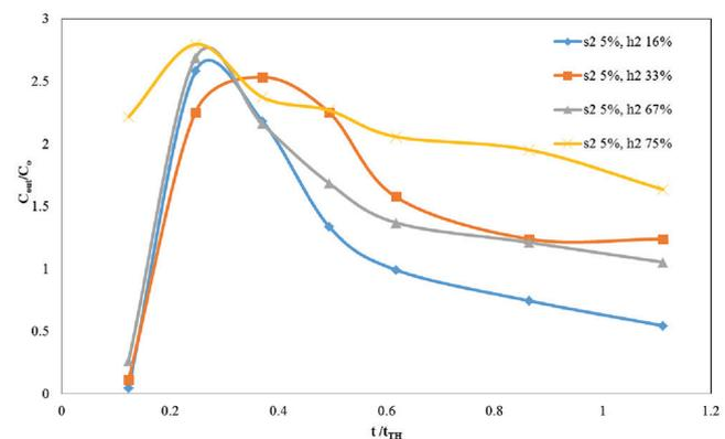
Fig. 12. Time of maximum concentration for different outlet baffle vertical position (h2 = 16%, 33%, 65% and 75; and s2 = 5% of the length).
