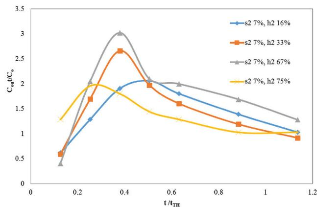
Fig. 14. Time of maximum concentration for different outlet baffle vertical positions (h2 = 16%, 33%, 65% and 75; and s2 = 7% of the length).
