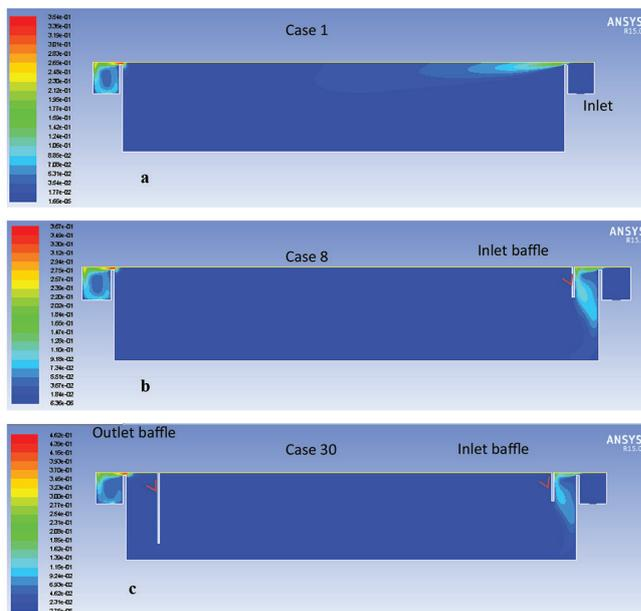
Fig. 18. Computed contour of kinetic energy at no baffle (a) Case (1), (b) inlet baffle Case (8), (c) inlet and outlet baffle Case (30).
