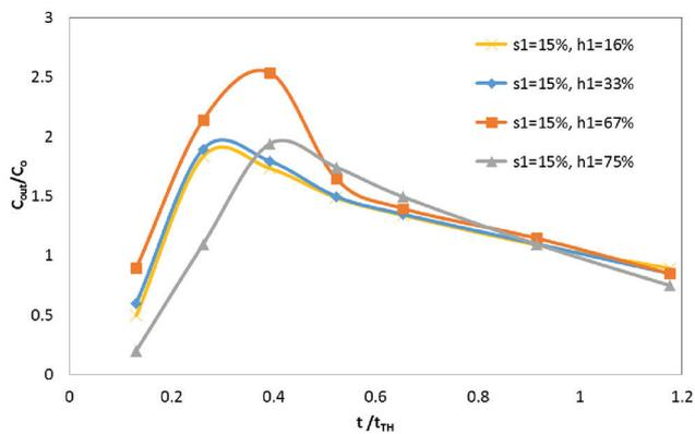
Fig. 9. Time of maximum concentration for different inlet baffle vertical positions (h1 = 16%, 33%, 65%, 75%; and s1 = 15% of the length).
