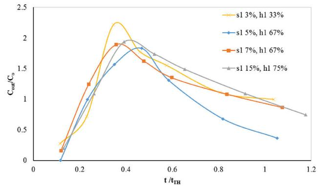
Fig. 10. Comparison between different inlet baffle best longitudinal and vertical positions.
