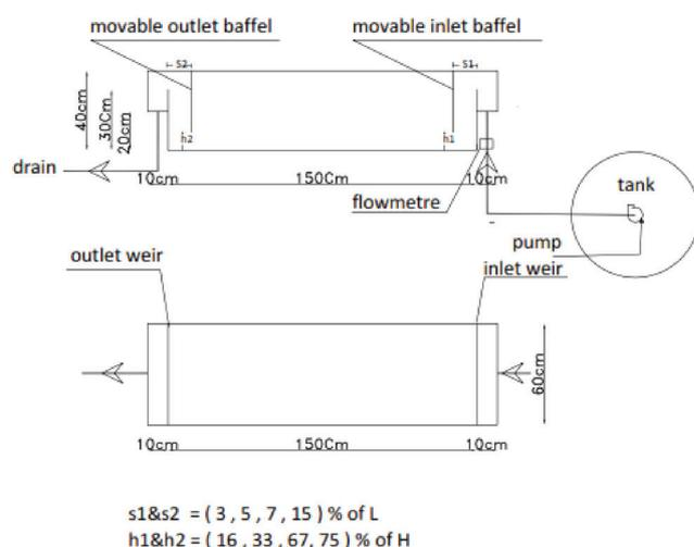
Fig. 2. Schematic diagram for pilot-scale sedimentation tank.
