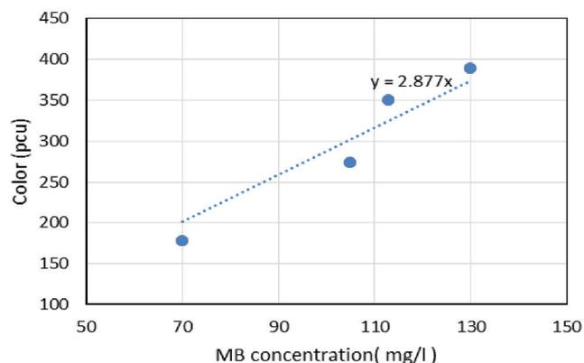
Fig. 3. Relation between colour concentration and Methylene blue concentration.
