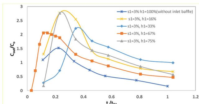
Fig. 5. Time of maximum concentration for different inlet baffle vertical positions (h1 = 16%, 33%, 67%, 75%, without baffle; and s1=3% of the length).
