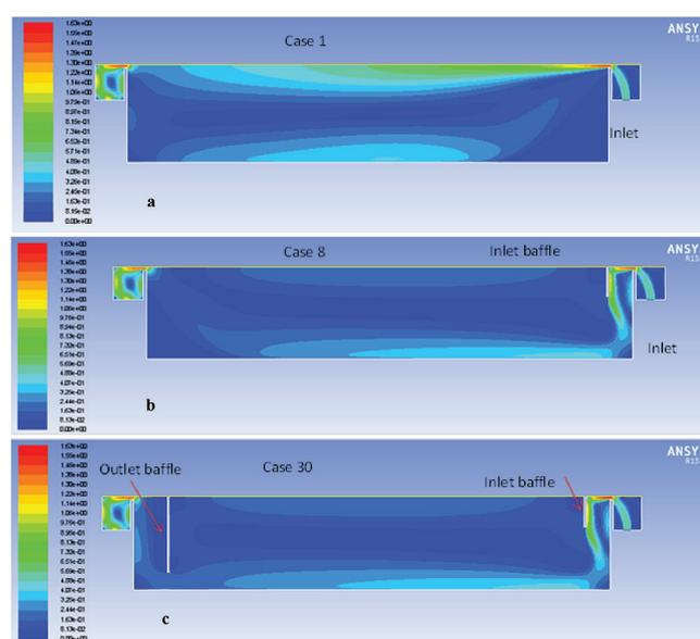
Fig. 17. Computed velocity vector contours at no baffle (a) Case (1), (b) inlet baffle Case (8), (c) inlet and outlet baffle Case (30).
