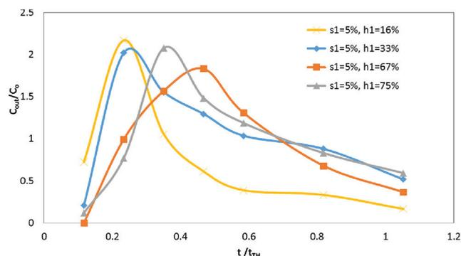
Fig. 6. Time of maximum concentration for different inlet baffle vertical position (h1 = 16%, 33%, 65%, 75%; s1 = 5% of the length).
