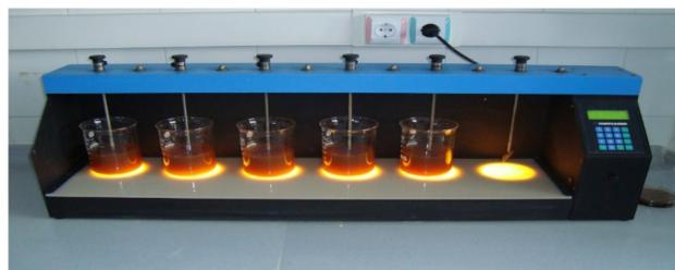
Fig. 1. Schematic view of the experimental system for the lab-scale Fenton oxidation treatment of PPIW.
