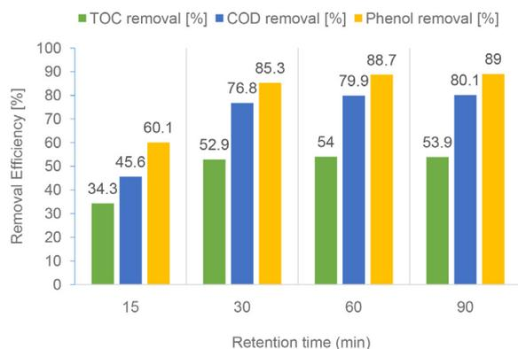
Fig. 5. The effect of the reaction time on the TOC, COD, and phenol removal (1.32  $g\ L^{-1}\ Fe^{2+}$ , 19.2  $g\ L^{-1}\ H_2O_2$ , and initial PPIW pH = 3).
