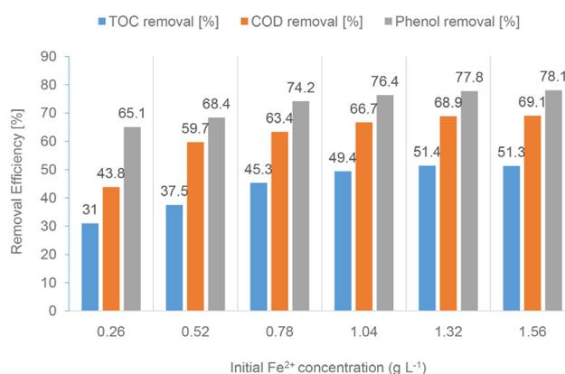
Fig. 2. Effect of different initial  $\text{Fe}^{2+}$  concentrations on the TOC, COD, and phenol removal (19.2  $\text{g L}^{-1}$   $\text{H}_2\text{O}_2$ , initial PPIW pH = 5.2, and reaction time = 60 min).
