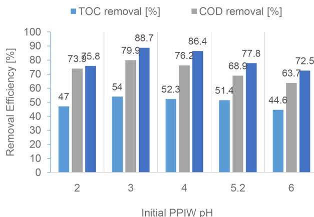
Fig. 4. The effect of different PPIW initial pH on TOC, COD, and phenol removal (1.32  $g\ L^{-1}\ Fe^{2+}$ , 19.2  $g\ L^{-1}\ H_2O_2$ , and reaction time = 60 min).
