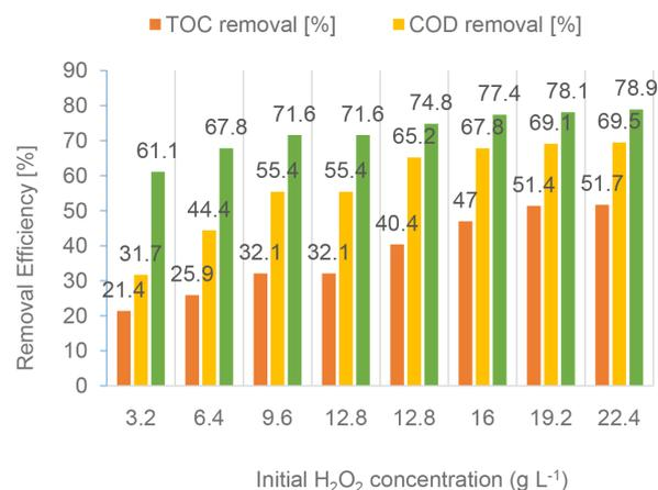
Fig. 3. The effect of different initial H<sub>2</sub>O<sub>2</sub> concentrations on the TOC, COD, and P removal (1.32 g L<sup>-1</sup> Fe<sup>2+</sup>, initial PPIW pH = 5.2, and reaction time = 60 min).
