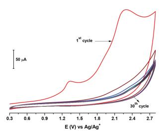
Fig. 2. Cyclic voltammogram of 1 mM HMPD in 100 mM NBu $_4$ BF $_4$  (in CH $_3$ CN) vs. Ag/Ag $^+$ /(10 mM AgNO $_3$ ) on bare GC electrode surface. Potential range from +300 to +2,800 mV, sweep rate is 100 mV s $^{-1}$  and 30 cycles.
