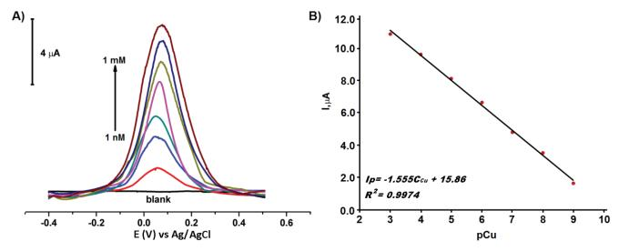
Fig. 8. (A) Differential pulse voltammograms of different concentrations of standard Cu(II) solution changing from  $1.0 \times 10^{-9}$  to  $1.0 \times 10^{-3}$  M (from 1,000 ppm stock solution) (BR buffer, pH 5.0) solution on HMPD/GC. The measurements were performed in BR buffer solution, pH 5.0, vs. Ag/AgCl/(3 M KCl). Sweep rate was 50 mV s<sup>-1</sup>. (B) Linear relationship between peak currents and different concentrations of Cu(II) ions.
