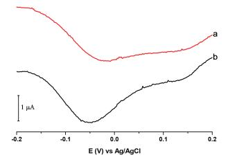
Fig. 9. Differential pulse voltammogram of Cu(II) ions in (a) flour sample and (b) water sample on the HMPD/GC electrode surfaces. The measurement was performed in BR buffer, pH 5.0, potential is referred vs. Ag/AgCI/(3 M KCl).
