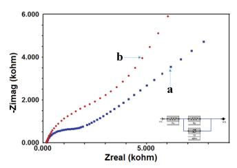
Fig. 5. Nyquist plots of 1 mM of  $Fe(CN)_6^{3-}/Fe(CN)_6^{4-}$  in 0.1 M of KCl of bare GC (a), and HMPD/GC electrode (b). Frequency range is from 100.000 to 0.05 Hz, the modulation amplitude is 10 mV. Inset: equivalent circuit applied for calculations.
