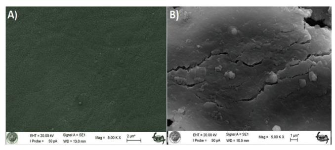
Fig. 6. SEM images of (A) bare GC and (B) HMPD/GC electrode surfaces.
