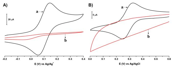
Fig. 4. Overlaying the bare GC and HMPD/GC voltammograms (A) 1 mM ferrocene redox probe solution vs.  $Ag/Ag^+$  (10 mM) in MeCN + 0.1 M NBu<sub>4</sub>BF<sub>4</sub>, (a) bare GC and (b) HMPD/GC; (B) 1 mM Fe(CN)<sub>6</sub><sup>3-</sup> redox probe solution vs. Ag/AgCl/(3 M KCl) in BR buffer solution, pH 2.0, (a) bare GC and (b) HMPD/GC. Sweep rate was 100 mV s<sup>-1</sup>.
