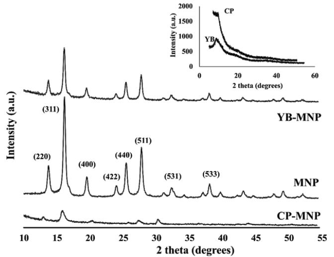
Fig. 2. Powder X-ray diffractograms from CP (cork powder), CP-MNP (ferromagnetic nanocomposites of cork powder), YB (yeast biomass), YB-MNP (ferromagnetic nanocomposites of yeast biomass), and MNP (magnetite nanoparticles), displaying the Bragg peak reflections of magnetite for the magnetic adsorbents.
