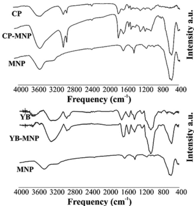
Fig. 4. FTIR spectra of CP (cork powder), CP-MNP (ferromagnetic nanocomposites of cork powder), YB (yeast biomass), MNP-YB (yeast magnetic bionanocomposite), and MNP (magnetic nanoparticles).
