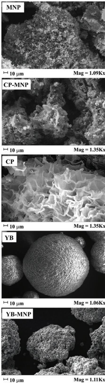
Fig. 1. SEM images of CP (cork powder), CP-MNP (ferromagnetic nanocomposites of cork powder), YB (yeast biomass), YB-MNP (ferromagnetic nanocomposites of yeast biomass), and MNP (magnetite nanoparticles).
