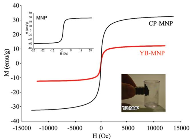
Fig. 3. Susceptibility of magnetization curves for CP-MNP (ferromagnetic nanocomposites of cork powder), YB-MNP (ferromagnetic nanocomposites of yeast biomass), and MNP (magnetite nanoparticles) and an illustrative picture of YB-MNP being attracted by a magnet.
