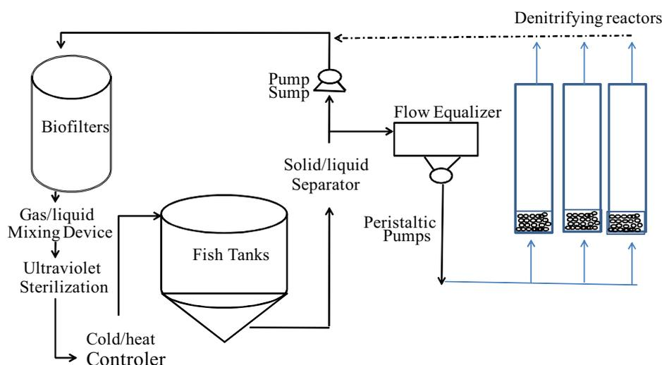
Fig. 1. Schematics of three pilot-scale PCL-packed reactors for treating nitrate-dosed water from a recirculating aquaculture system.
