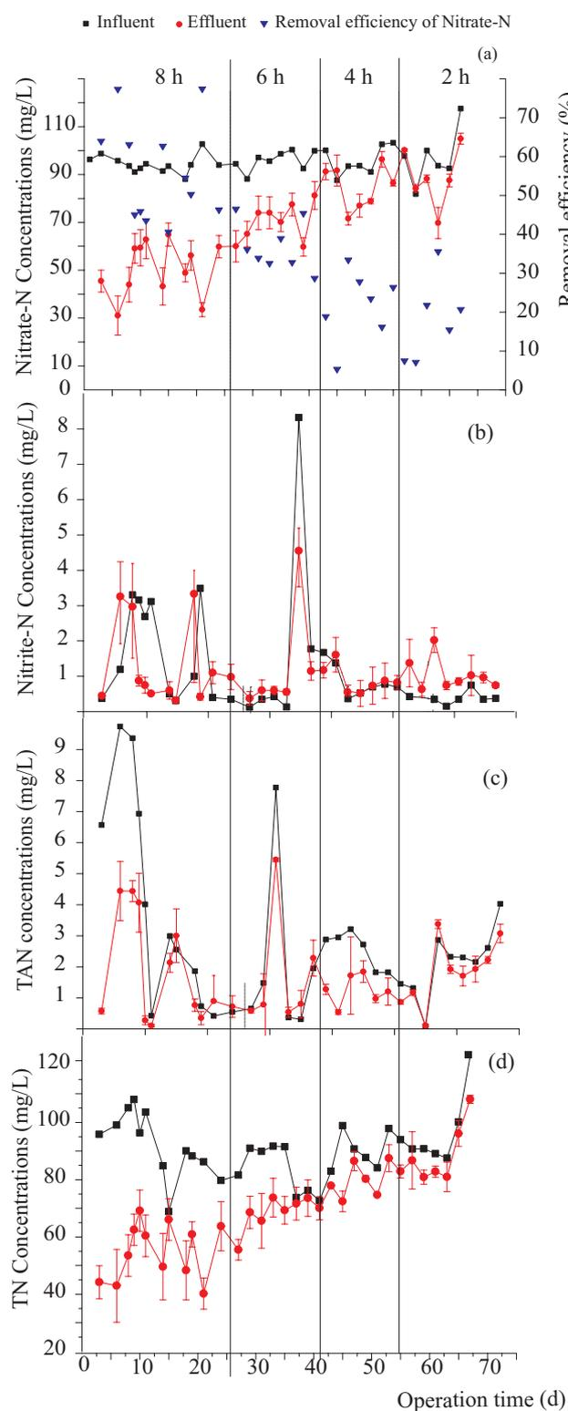
Fig. 2. Influent and effluent  $\text{NO}_3^-$ -N (a),  $\text{NO}_2^-$ -N (b), total ammonia nitrogen (TAN, c), and total nitrogen (TN, d) from pilot PCL-packed reactors that treated nitrate-dosed water from a recirculating aquaculture system. The hydraulic retention time (HRT) of the reactors is indicated in the figure in hours.
