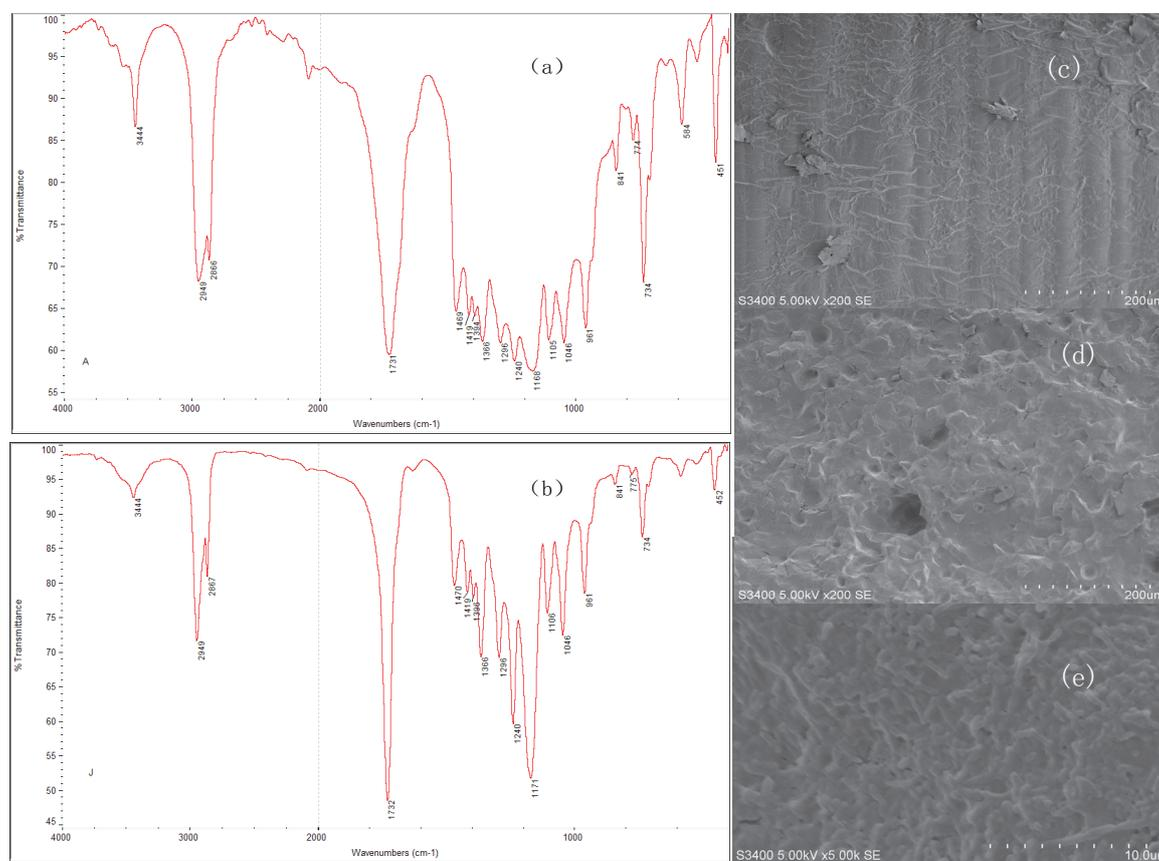
Fig. 6. FT-IR spectra of fresh PCL (a), used PCL (b), SEM observations of the surface of fresh PCL (c), PCL after biofilm detachment (d), and the biofilm attached to PCL (e) at the end of the experiment.
