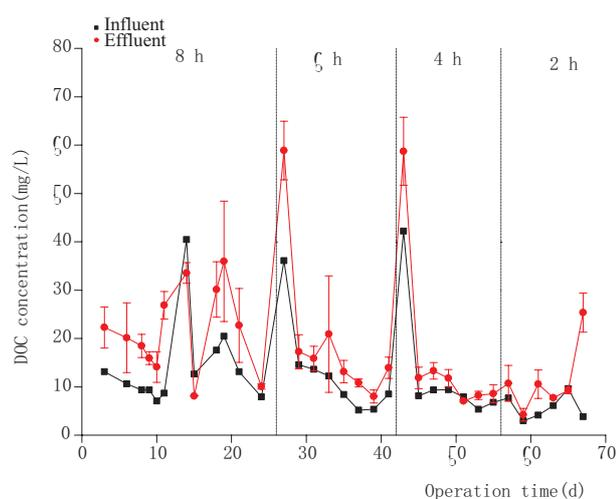
Fig. 3. Influent and effluent dissolved organic carbon (DOC) from the pilot PCL-packed reactors treating nitrate-dosed water from a recirculating aquaculture system. The reactor hydraulic retention time (HRT) is indicated in the figure in hours.
