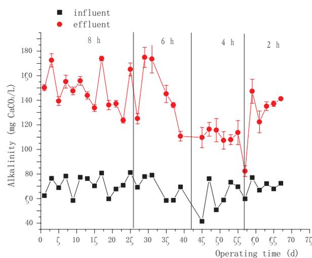
Fig. 4. Alkalinity (ALK) of the influent and effluent of pilot PCL-packed reactors treating nitrate-dosed water from a recirculating aquaculture system. The reactor hydraulic retention time (HRT) is indicated in the figure in hours.
