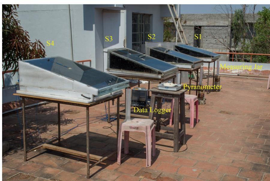
Fig. 3. Photograph of the experimental set up.
