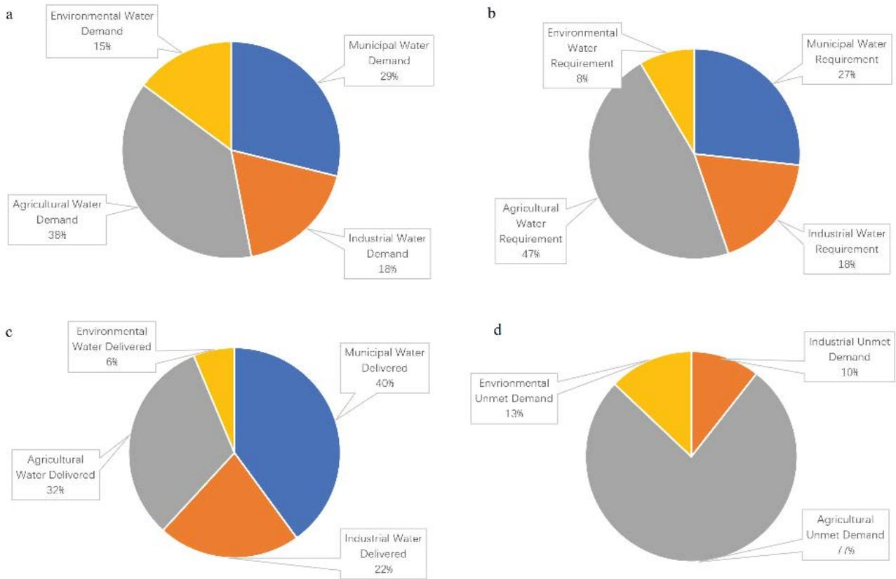
Fig. 6. Water supply and demand calculated by Beijing WEAP 2010. (a) water demands; (b) water requirements; (c) supply delivered; (d) unmet demands.
