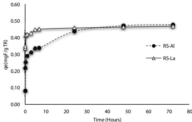
Fig. 3. Contact time versus sorption capacity of fluoride (0.1 g of sorbent in 10 mL of fluoride solution).
