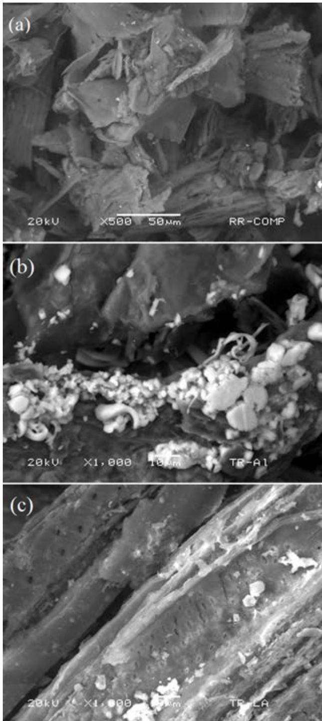
Fig. 1. SEM images of (a) undoped stems of rose, (b) stems of rose doped with aluminum, and (c) stems of rose doped with lanthanum.
