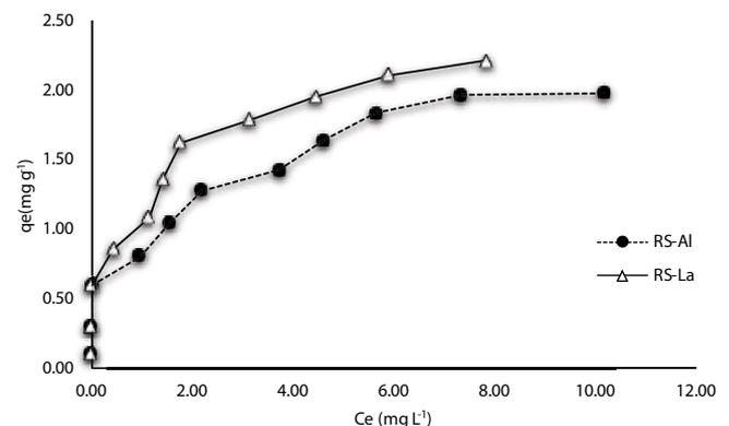
Fig. 4. Sorption isotherm of fluoride ions by SR-Al or SR-La.
