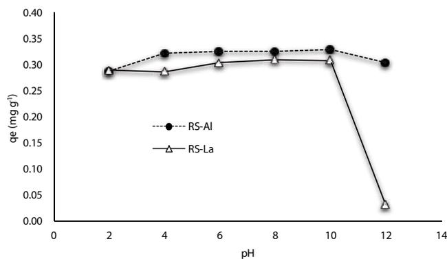
Fig. 5. Effect of pH on the removal of fluoride ions by RS-Al or RS-La.
