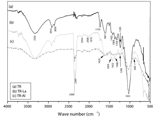
Fig. 2. FTIR spectra of stem of rose before and after doped with La or Al.
