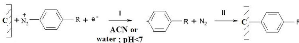
Fig. 2. Scheme of aryl diazonium salt reduction on coal surface.
