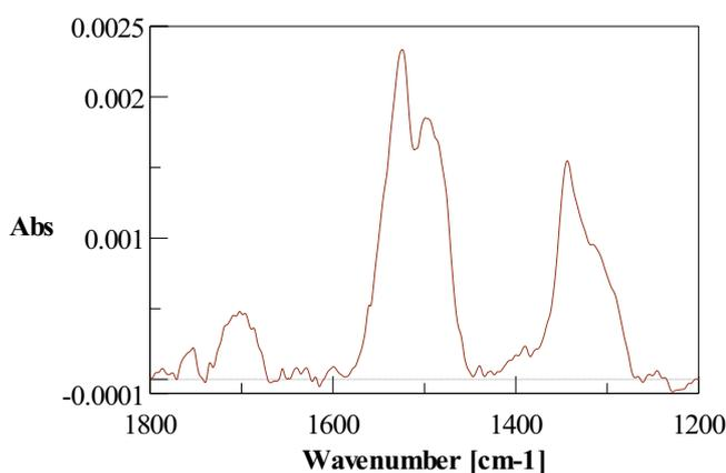
Fig. 1. ATR-FTIR spectra of modified coal with nitrophenyl groups in H<sub>3</sub>PO<sub>2</sub> (0.01 M).
