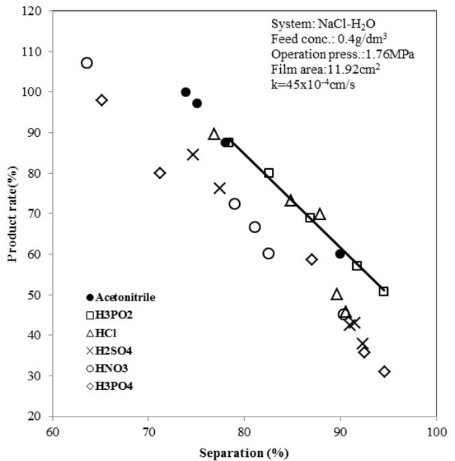
Fig. 4. Product rate and solute separation results of RO membranes (batch 317K-1, IV) made with modified coal particles of DS (20 mM) in different aqueous acidic mediums of the same concentration 0.01 M and acetonitrile.
