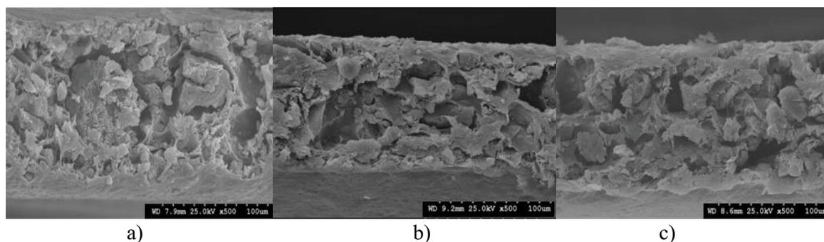
Fig. 5. SEM images of HAROM membranes: (a) batch 317K-1 II, (b) batch 317K-1 III, and (c) batch 317K-1 IV in aqueous acid medium ( $\text{H}_3\text{PO}_2$  0.01 M).
