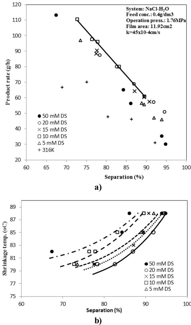
Fig. 3. (a) Product rate and solute separation results of RO membranes made with modified coal particles at different concentrations of aryl diazonium salts: batches 317K-1, I; II; III; IV; and V and (b) shrinkage temperature versus solute separation.
