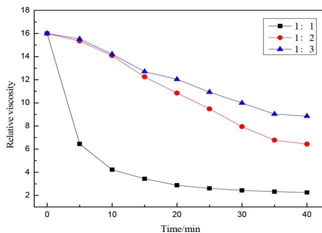
Fig. 5. Effect of metal-1,2-benzenediol complex ratio on the degradation.
