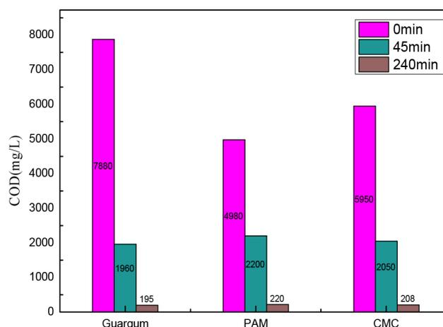
Fig. 13. COD removal of Ni(II)L catalyzed oxidation for different polymers.
