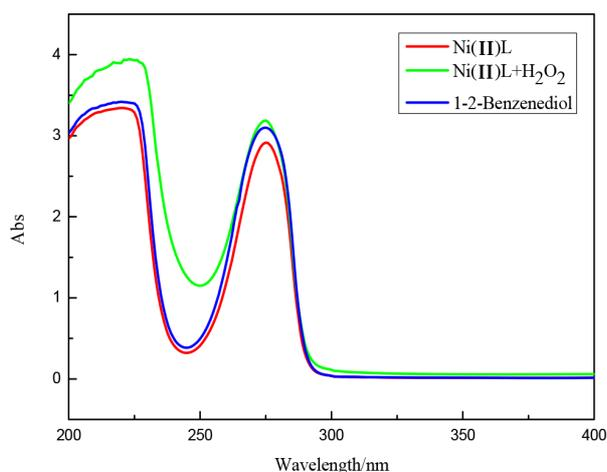
Fig. 12. UV spectra of ligand corresponding Ni(II) complex.
