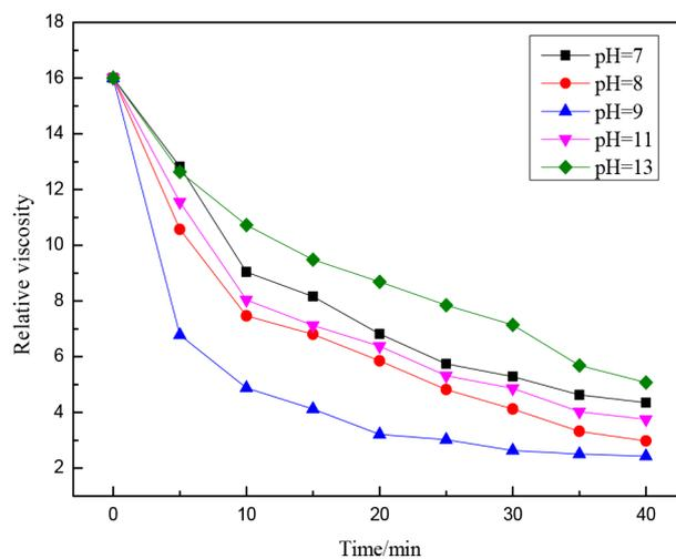
Fig. 11. Effect of pH value on the degradation.
