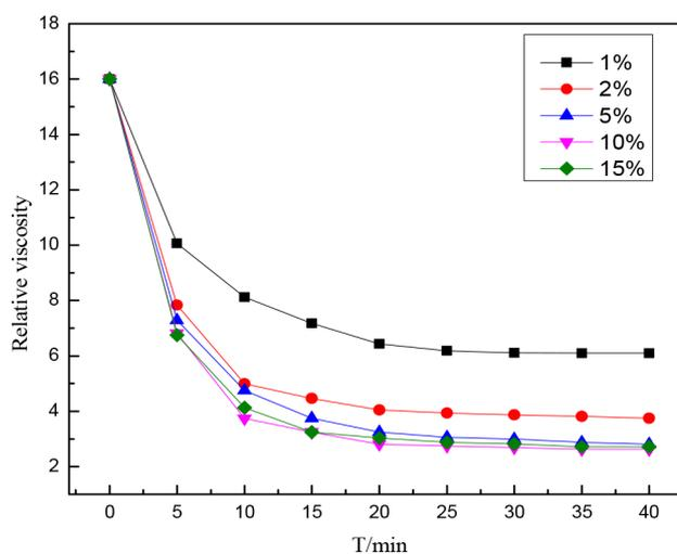
Fig. 8. Effect of molar ratio of hydroxypropyl guar gum/ $\text{H}_2\text{O}_2$ .
