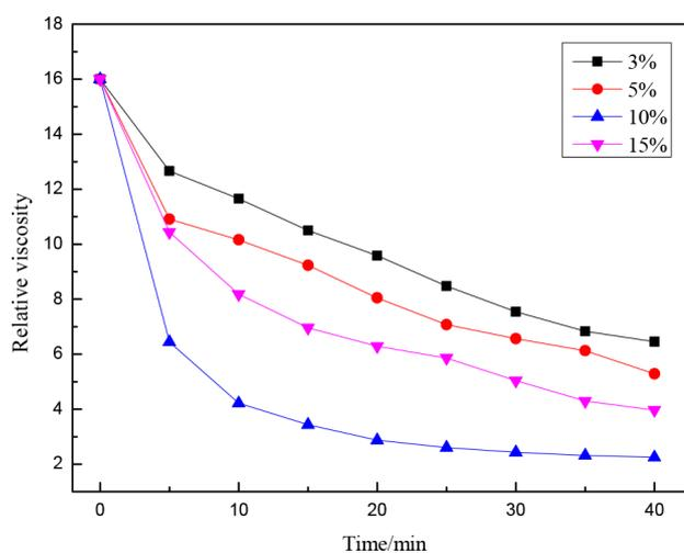
Fig. 7. Effect of different amount of catalyst on the degradation.
