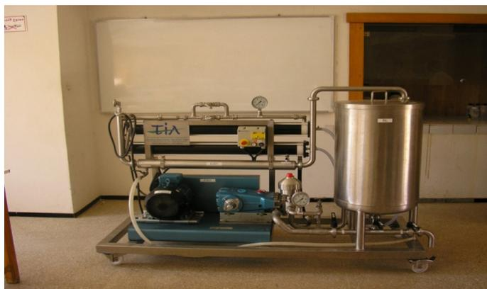
Fig. 1. Schematic diagram and picture of the nanofiltration/reverse osmosis pilot plant. T: tank; P: feed pump; V: pressure regulation valves; M: nanofiltration module; Pe: permeate recirculation; R: retentate recirculation; H: heat exchanger; 1: pressure sensor; 2: temperature sensor.
