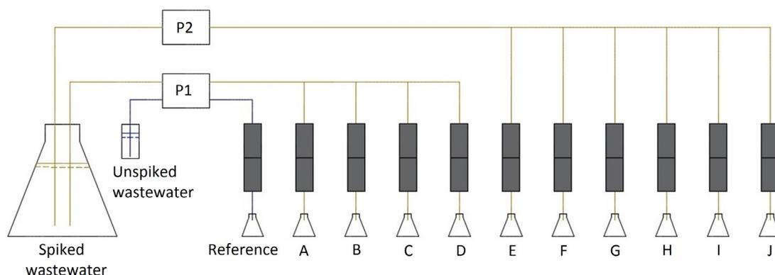
Fig. 1. Schematic of the column experiment including five organic and five inorganic sorbents (note: not to scale). Name of the sorbents (from left to right): (A) Filtrasorb<sup>®</sup>300, (B) sand, (C) Xylit, (D) Filtra<sup>®</sup>N, (E) lignite, (F) Filtralite<sup>®</sup>P, (G) Zugol<sup>®</sup>, (H) Sorbulite<sup>®</sup>, (I) Envirocarb<sup>™</sup> 207EA, (J) Polonite<sup>®</sup>.
