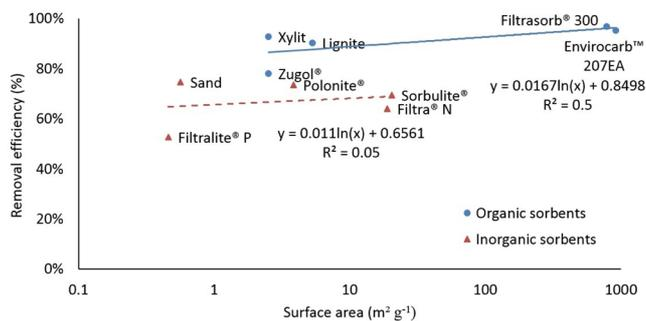
Fig. 6. Relationship between average removal efficiency of the analyzed MPs ( $n = 19$ ) and sorbent surface area of the tested materials ( $n = 10$ ).
