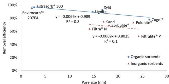
Fig. 5. Relationship between average removal efficiency of the analyzed MPs ( $n = 19$ ) and sorbent pore size of the tested materials ( $n = 10$ ).
