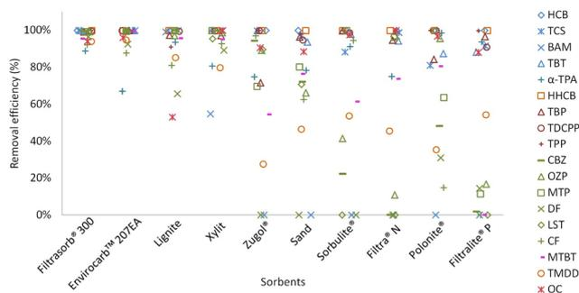
Fig. 3. Average removal efficiency (%) of individual MPs by the 10 sorbents.
