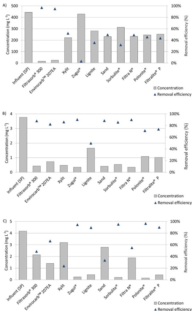
Fig. 2. Mean concentration of three wastewater quality parameters for two weeks: (A) dissolved organic carbon (DOC); (B) ammonium-nitrogen (NH<sub>4</sub>-N); (C) total phosphorus (P<sub>tot</sub>) in the spiked influent and in effluent from the 10 sorbents during two weeks of the experiment. The removal efficiency (RE) at the end of the experiment is shown as blue triangles.
