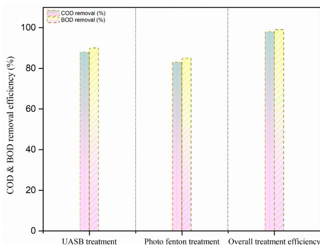
Fig. 7. Plot showing the overall treatment efficiency of the combined UASB and photo-Fenton treatment.
