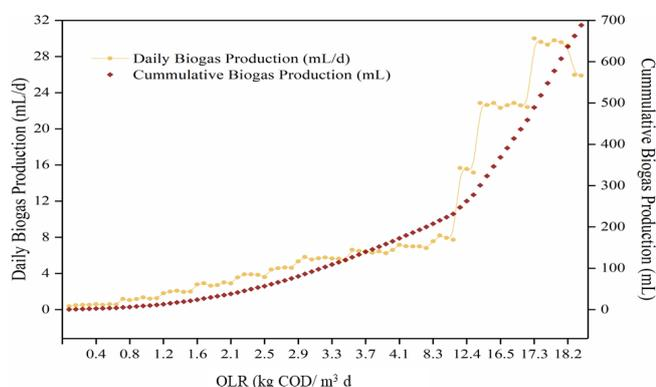
Fig. 4. Plot showing the biogas production during biological treatment of chocolaterie wastewater.
