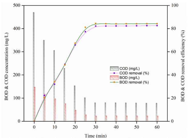
Fig. 6. Plot showing the COD and BOD concentration with its removal efficiency during photo-Fenton treatment of biologically treated chocolaterie wastewater.
