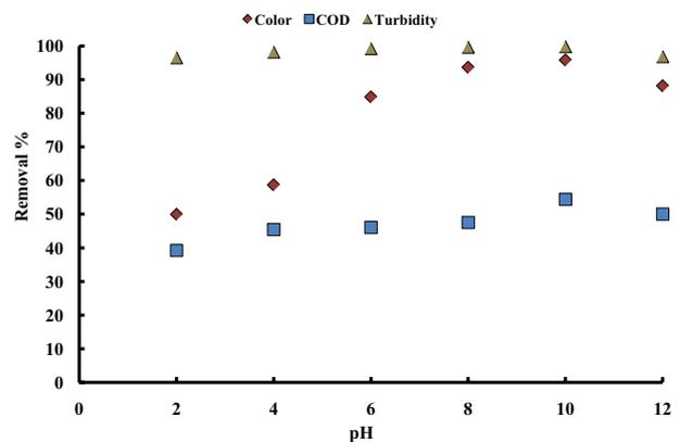
Fig. 6. Effect of pH on textile wastewater treatment.
