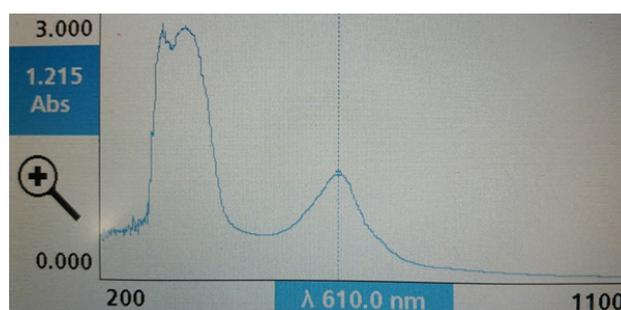
Fig. 1. UV-Vis absorption spectrum of industrial wastewater with maximum absorption at 610 nm.
