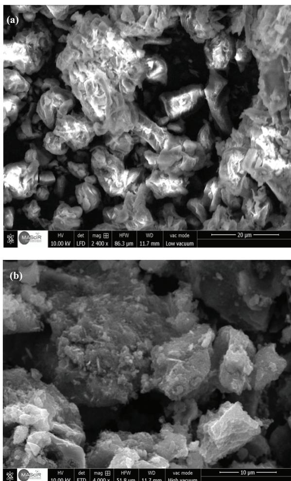
Fig. 2. Scanning electron micrographs of synthesized activated carbon (a)  $\times 2,400$  and (b)  $\times 4,000$ .
