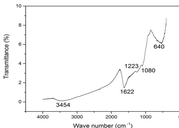
Fig. 4. FTIR spectrum of activated carbon from *Ziziphys lotus*.
