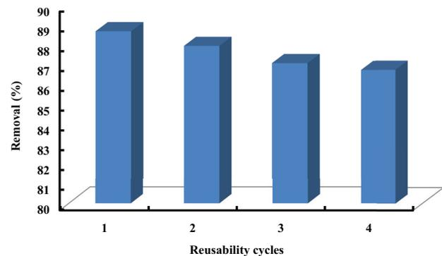
Fig. 9. Adsorption ability of the *Ziziphus lotus* activated carbon toward industrial wastewater at different cycles.
