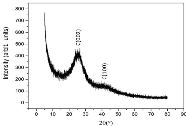
Fig. 5. XRD spectrum of activated carbon from *Ziziphus lotus*.
