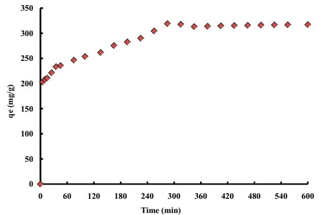
Fig. 8. Effect of contact time on textile dye treatment.
