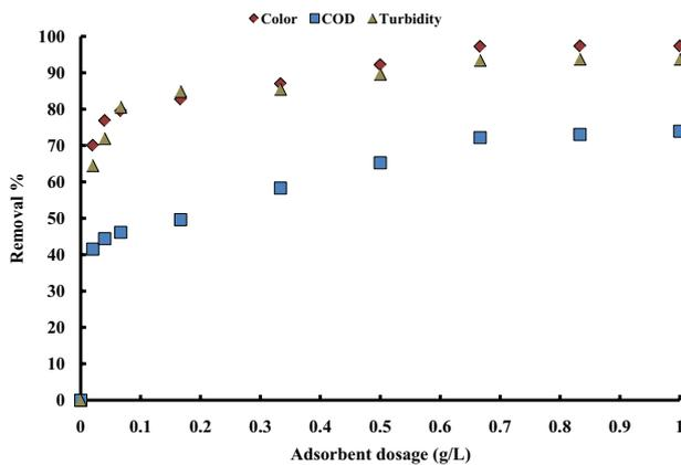
Fig. 7. Effect of adsorbent dosage on textile dye treatment.
