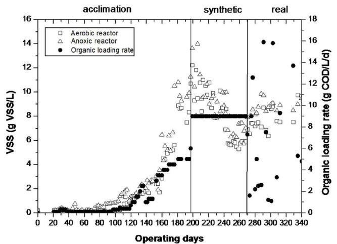
Fig. 2. VSS evolution in the reactors during MBR operation.
