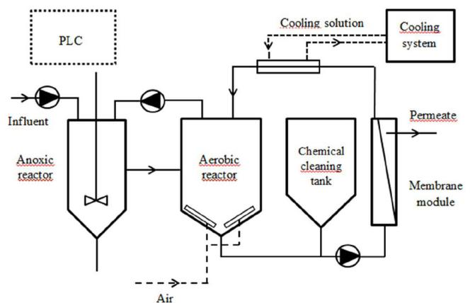
Fig. 1. Schematic representation of the laboratory-scale MBR.
