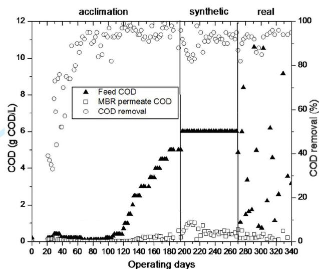
Fig. 4. MBR COD removal efficiency during operation period.
