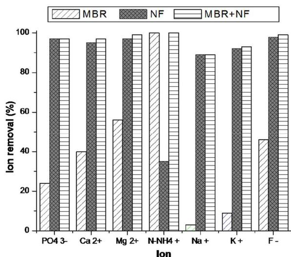
Fig. 5. Ion removal by MBR and NF.
