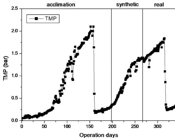
Fig. 6. TMP evolution over MBR operation.
