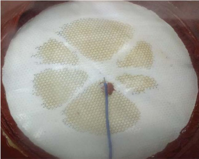
Fig. 6. Image of the pretested membrane after 3 h with detergent water.
