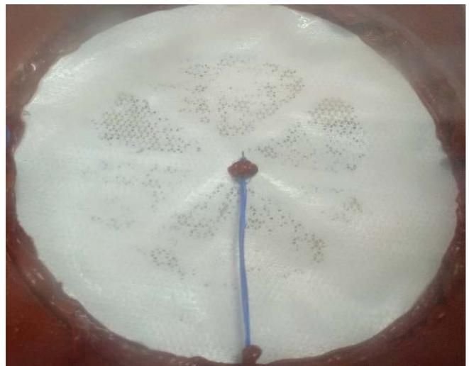
Fig. 5. Image of the fresh unused membrane after 20 min with detergent water.
