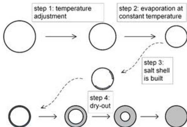
Fig. 7. The four steps of evaporation of saltwater in cooling towers according to Sadafi et al. [25].
