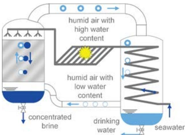
Fig. 1. HDH technology for desalination.
