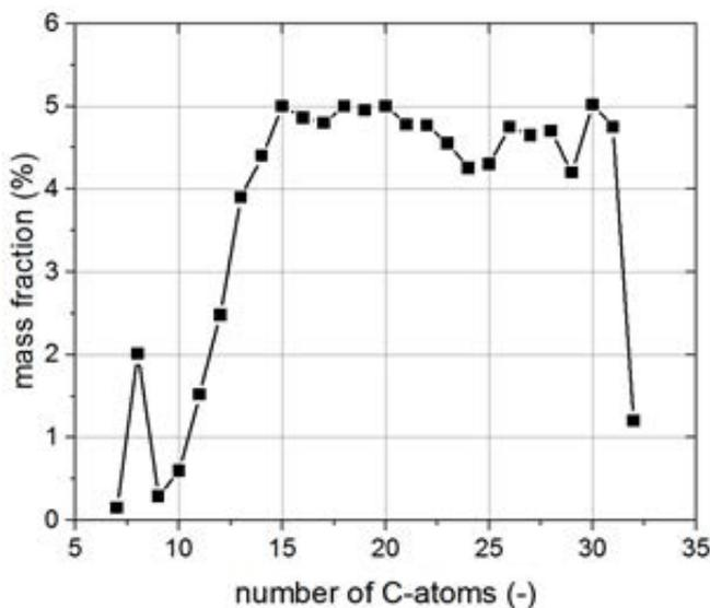
Fig. 9. Analysis of bilge water by means of gas chromatography.
