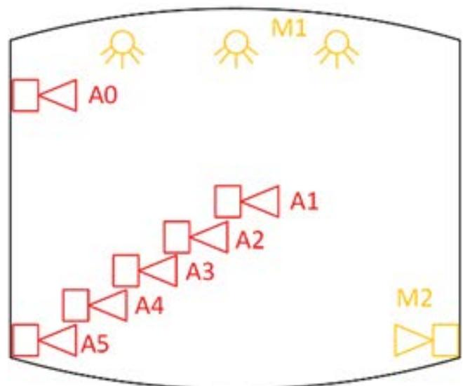
Fig. 5. Location and numbering of air nozzles (A) and medium nozzles (M).
