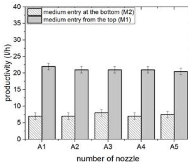
Fig. 11. Productivity for air entry in nozzle A1–A5 (striped: medium entry from bottom nozzle, gray: medium entry from top nozzle); mixture of 330 L of tap water and 190 L of bilge water.
