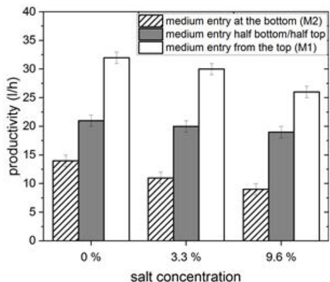
Fig. 8. Productivity for different salt concentrations with air entry from top (left: medium entry from bottom, middle: medium entry from top and bottom, right: medium entry from top).
