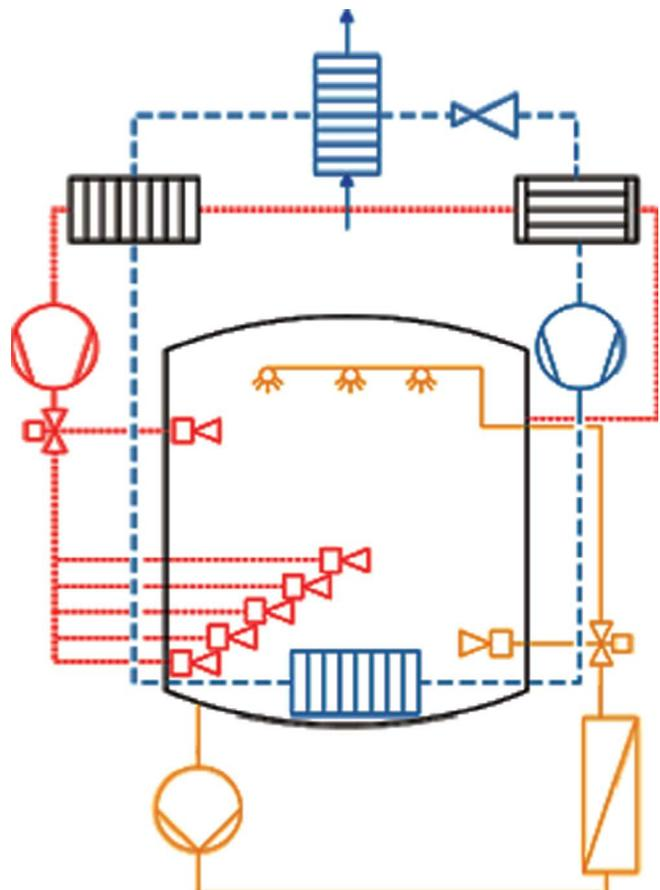
Fig. 2. Scheme of demonstration unit with heat pump cycle (dashed line, blue), air cycle (pointed line, red) and medium cycle (solid line, yellow).
