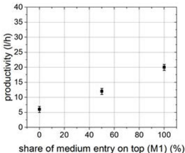
Fig. 12. Productivity depending on share of medium entry on top (M1); mixture of 330 L of tab water and 190 L of bilge water.
