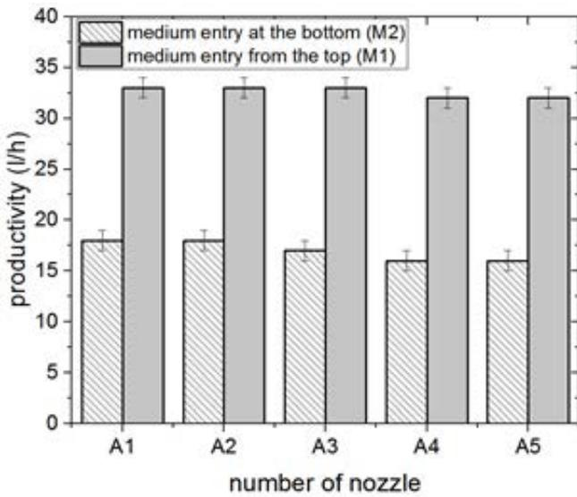
Fig. 6. Productivity for air entry in nozzle A1–A5 (striped: medium entry from bottom nozzle, gray: medium entry from top nozzle); salt concentration 0%.
