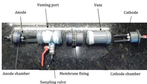
Fig. 3. Elements used in tested MFC.
