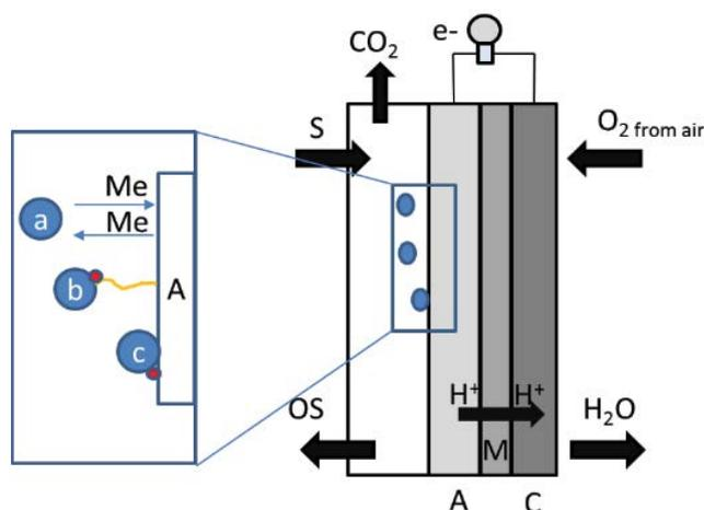
Fig. 2. Simplified scheme of two-chamber MFC with possible mechanisms of electron transfer: (a) electron transfer with the help of a mediator; (b) electron transfer with the help of nanowires, and (c) direct electron transfer with the help of external cell cytochromes.
