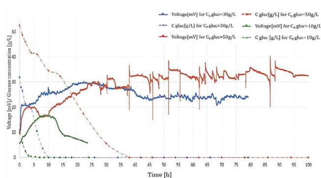
Fig. 5. Voltage and glucose concentration changes in time for the initial glucose concentrations in range 10–50 g/L (at the yeasts concentration 30 g/L).
