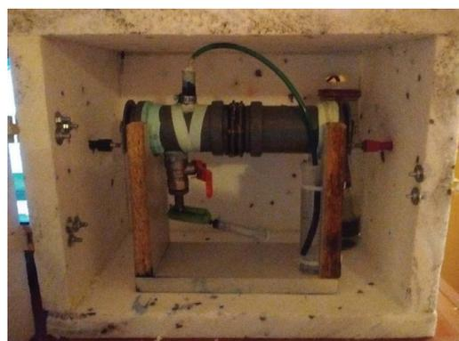
Fig. 4. Two-chamber MFC used in experiments.
