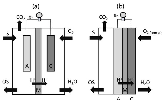
Fig. 1. Scheme of MFCs: (a) two-chamber, (b) one-chamber; S – substrate, OS – oxidized substrate, M – ion exchange membrane, A – anode, and C – cathode.
