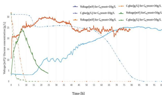
Fig. 6. Voltage and glucose concentration changes in time for the initial yeasts concentrations in range 10–50 g/L (for initial glucose concentration 30 g/L).
