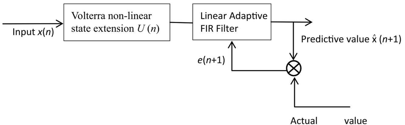
Fig. 1. Volterra adaptive filter structure.
