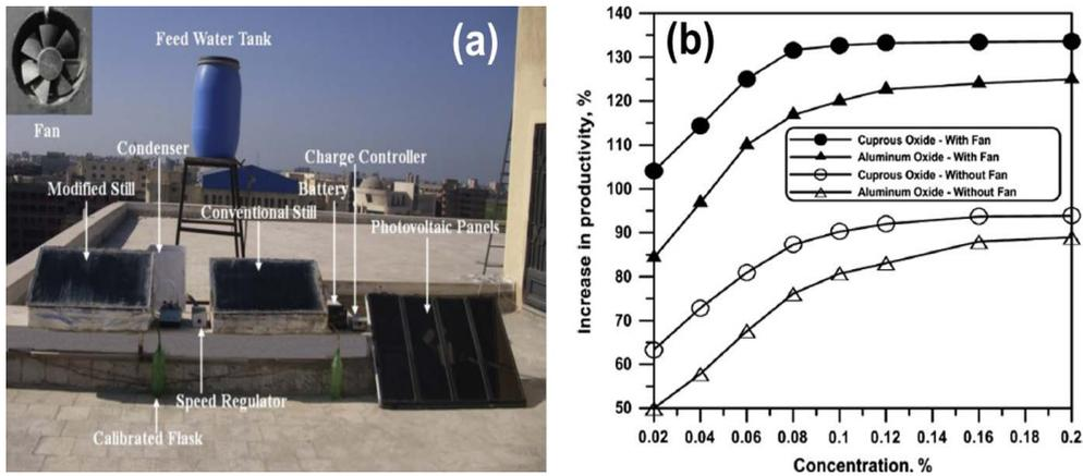
Fig. 6. (a) Pictorial view of experimental arrangement, and (b) effect of nanoparticle concentration [64].
