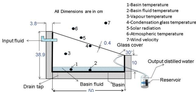
Fig. 9. Schematic diagram of solar still with basin fluid [67].
