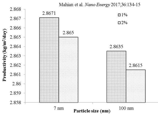
Fig. 17. Graphical view of productivity with respect to particle size [66].
