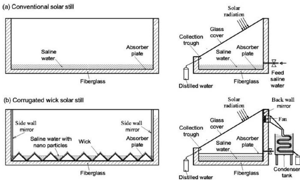
Fig. 7. Cross-sectional view of modified solar still with nanoparticles [65].
