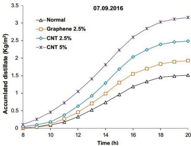
Fig. 13. Graphical view of pyramid solar still productivity [81].
