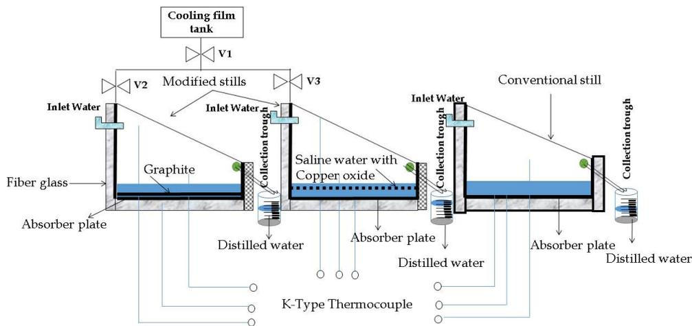
Fig. 12. SSSS with graphite microflakes and nanomaterial [77].
