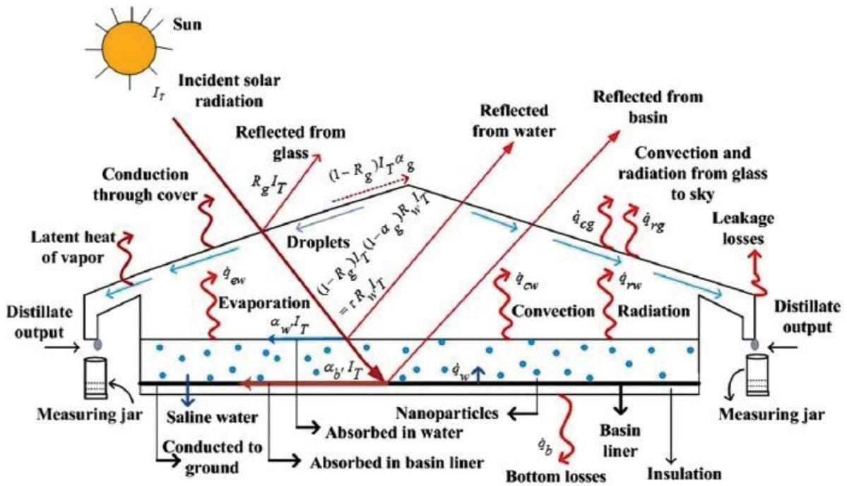
Fig. 1. Schematic view of double slope solar still with nanoparticles in the basin [59].
