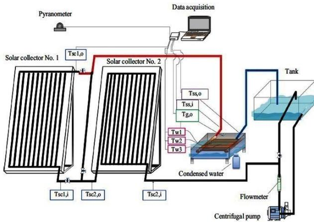
Fig. 8. SSSS integrated with FPC and heat exchanger coil [66].
