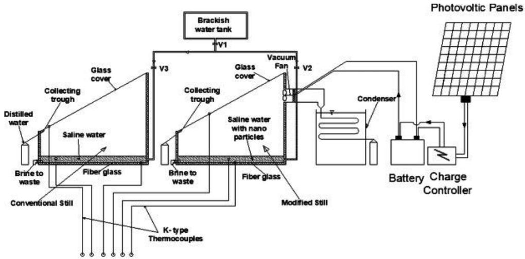
Fig. 5. Solar still with nanoparticles with external condenser [63].
