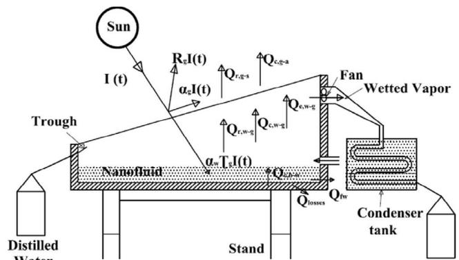
Fig. 4. SSSS with nanofluid in the basin [61].
