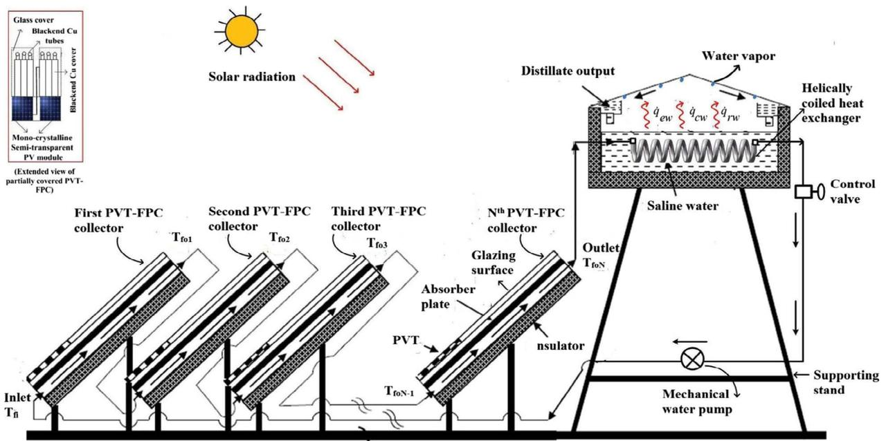
Fig. 2. Double slope solar still integrated with PVT-FPC [60].
