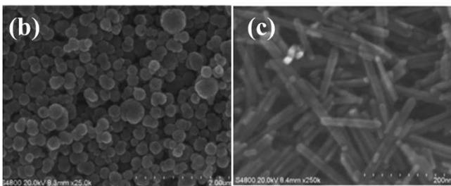
Fig. 10. (a) Tubular solar still, (b) ZnO spherical nanoparticles, and (c) ZnO nanorods [69].
