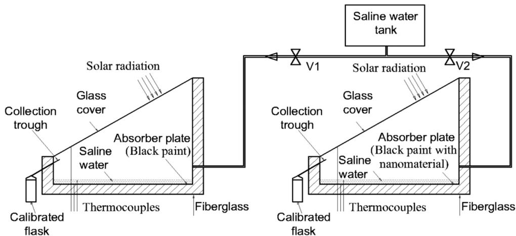
Fig. 11. Schematic view of solar still with nanomaterial [75].
