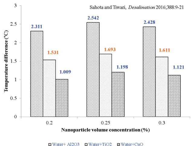
Fig. 15. Graphical view of temperature difference with respect to volume concentration [59].
