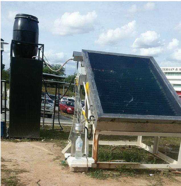
Fig. 3. The developed inclined copper-stepped solar still with the main components.
