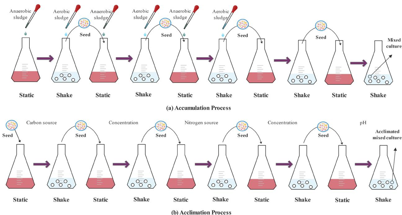
Fig. 1. The procedure of anoxic-aerobic circle accumulation process (a) and acclimation process (b).
