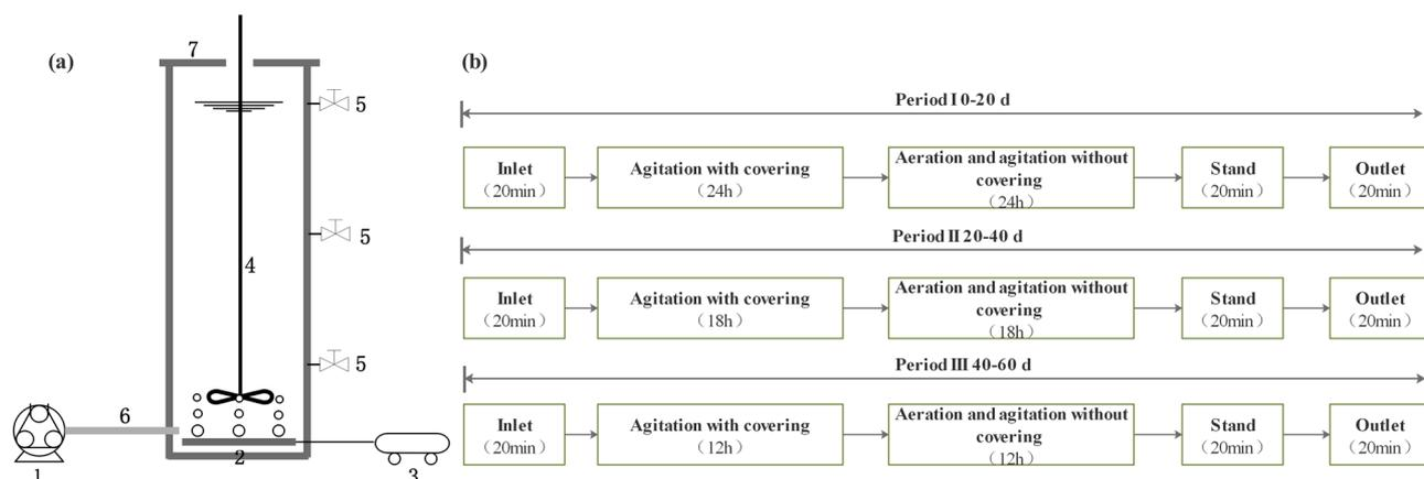
Fig. 2. Schematic structure (a) and operation method of SBR. 1: Peristaltic pump; 2: Aeration Heater; 3: Air pump; 4: Stirrer; 5: Outlet; 6: Inlet; 7: Covering.
