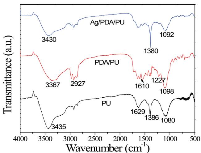
Fig. 2. FTIR spectra of PU sponge, PDA/PU sponge, and Ag/PDA/PU sponge.
