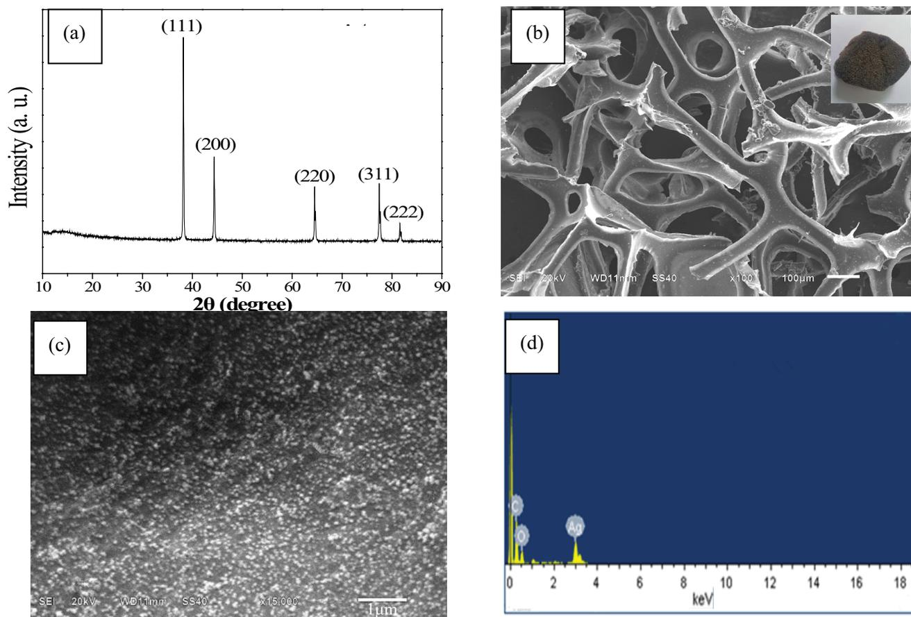
Fig. 1. XRD of Ag/PDA/PU sponge (a), SEM of Ag/PDA/PU sponge (b), an enlarged view of (figure b) (c), and EDS spectrum of Ag/PDA/PU sponge (d).
