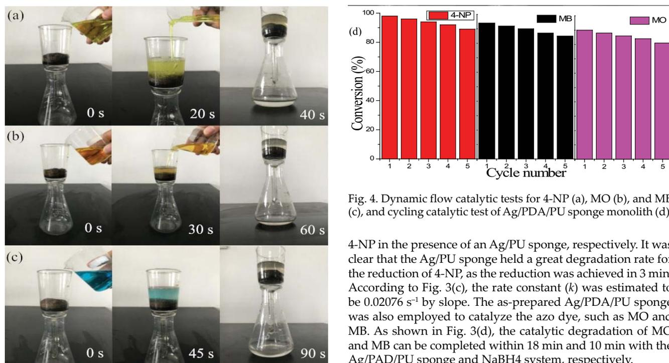
Fig. 4. Dynamic flow catalytic tests for 4-NP (a), MO (b), and MB (c), and cycling catalytic test of Ag/PDA/PU sponge monolith (d).
