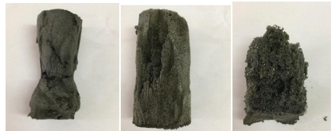
Fig. 2. Poor quality foam samples with activated carbon content greater than 5.81%.
