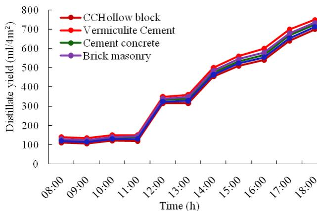
Fig. 4. Variation of distillate yield for different basin type of solar still during December 2017.
