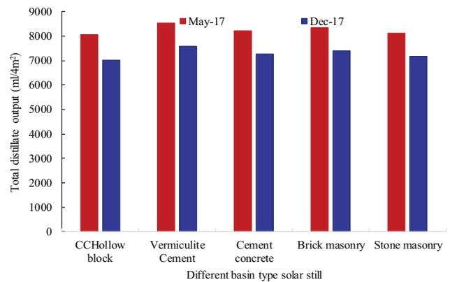
Fig. 5. Total distillate output including night for various basin type solar still.
