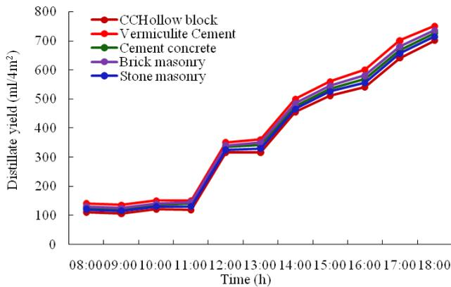
Fig. 3. Variation of distillate yield for different basin type of solar still during May 2017.
