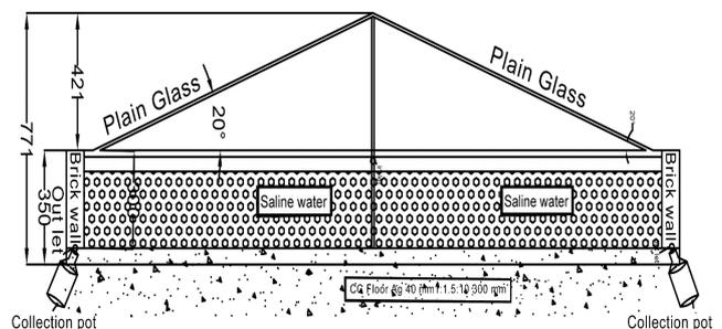
Fig. 1. Schematic diagram of basin type solar desalination device.
