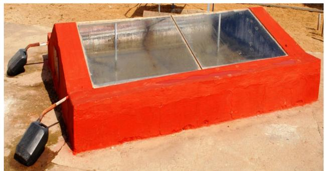
Fig. 2. Solar desalination devices made of vermiculite-cement plastered material.
