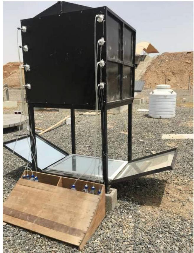
Fig. 2. Solar still setup and experiment using seawater in Muscat, Oman.
