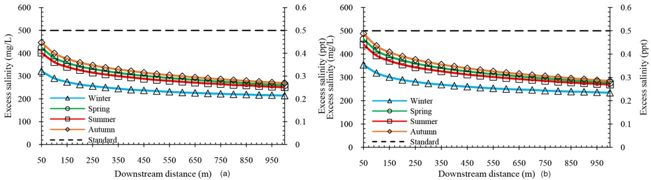
Fig. 10. Brine plume downstream dilution: (a) MSL; (b) LAT.
