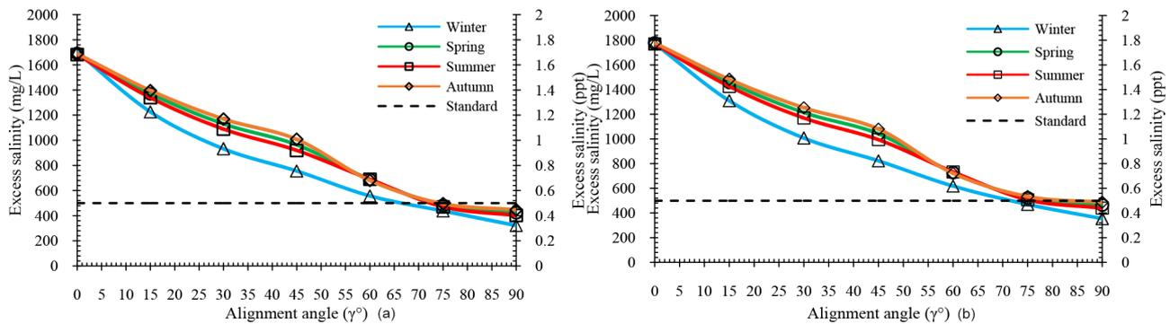
Fig. 11. Brine dilution as a function of alignment angle of diffuser within the RMZ: (a) MSL; (b) LAT.
