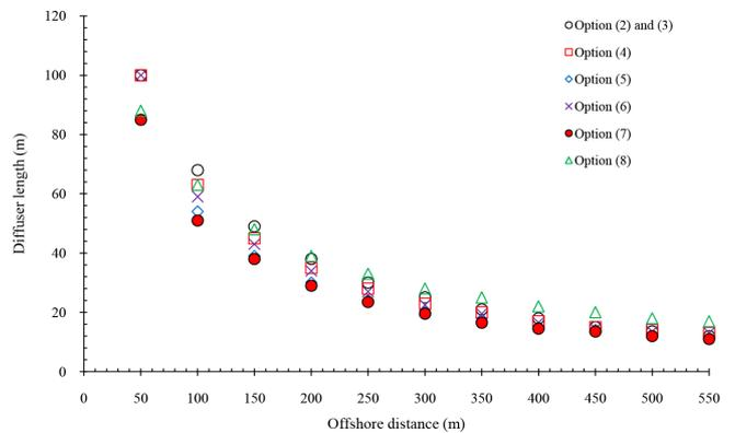
Fig. 9. Diffuser length as a function of offshore distance at RMZ.
