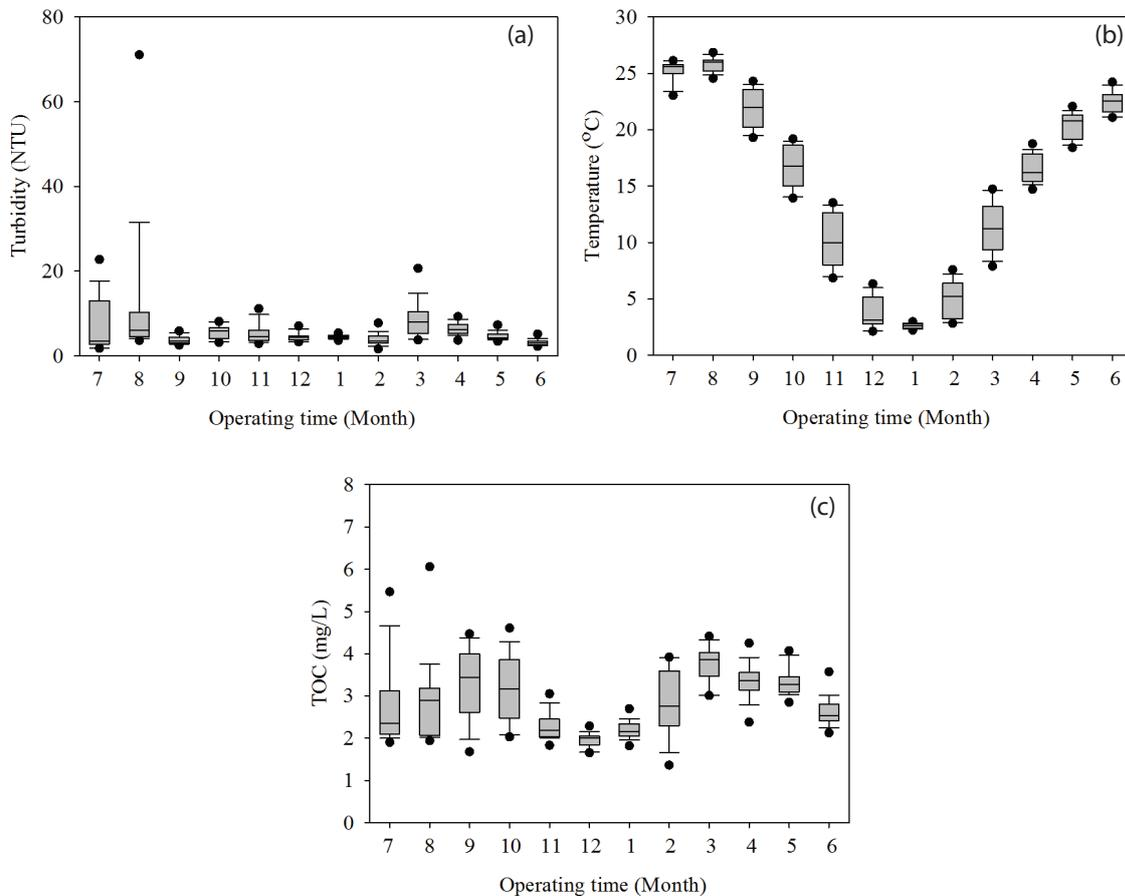
Fig. 3. Seasonal variations in the feed water quality: (a) turbidity (NTU), (b) temperature (°C) and (c) TOC (mg/L).
