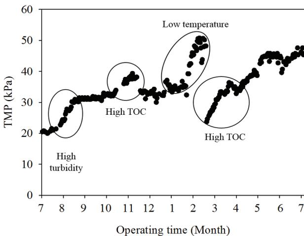
Fig. 4. Changes in TMP for pilot-scale submerged MF plant.
