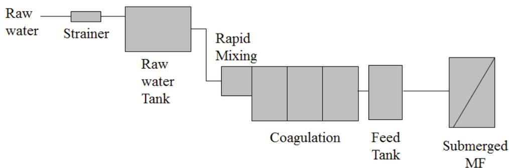
Fig. 2. Schematic diagram of the submerged MF pilot plant.
