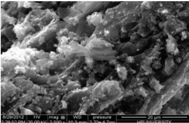
Fig. 2. Scanning electron microscope images of calcium alginate bead with zero valent iron (Fe<sup>0</sup>).
