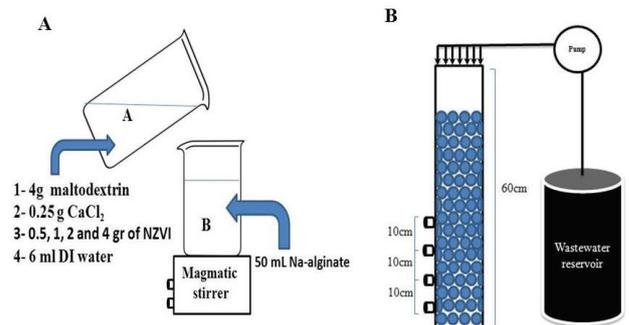
Fig. 1. (A) Preparation of Ca-alginate capsule. (B) The schematic of Ca-alginate column.
